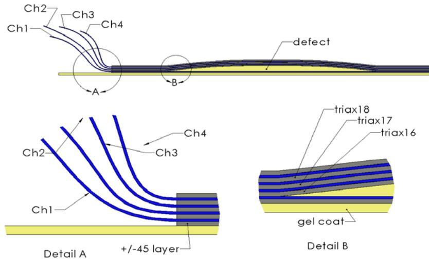
Figure 3: Sectional view of defect with optical fibers embedded between four layers of the spar cap [2].
