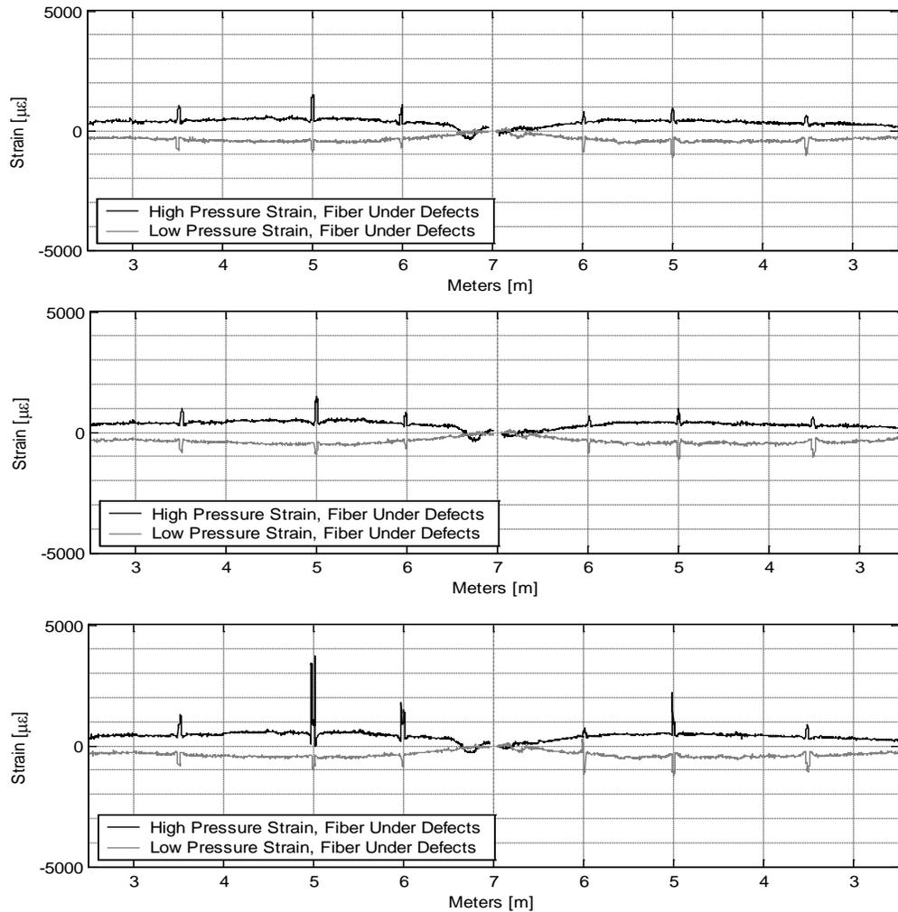
Figure 5: DFS embedded fibers located in +/- 45 layer under defects at 0 cycles (top), 204k cycles (middle), and 716k cycles (bottom). Note that the OBR identifies the failure point at less than half the cycles if took to actually achieve failure [3].
