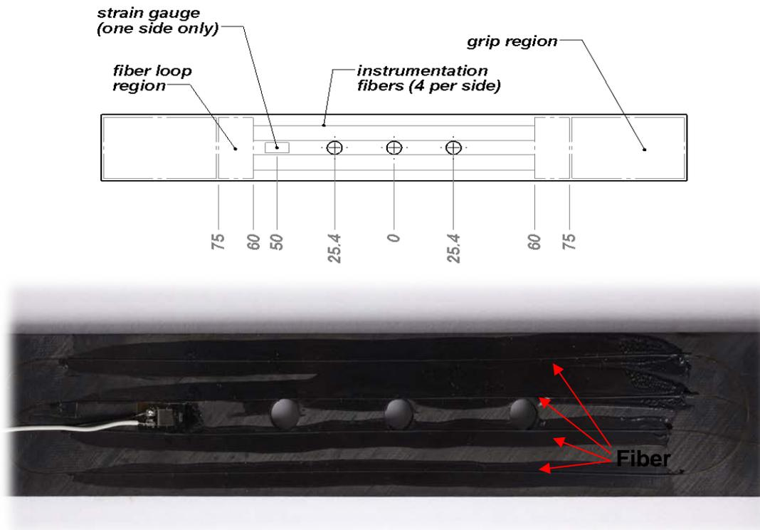
Figure 1: Depiction of a sample coupon cut from the composite panel. It features three open holes, an electrical foil strain gauge, and a surface bonded optical fiber. Measurements are in millimeters (top) [1]. A picture of the actual coupon (bottom).
