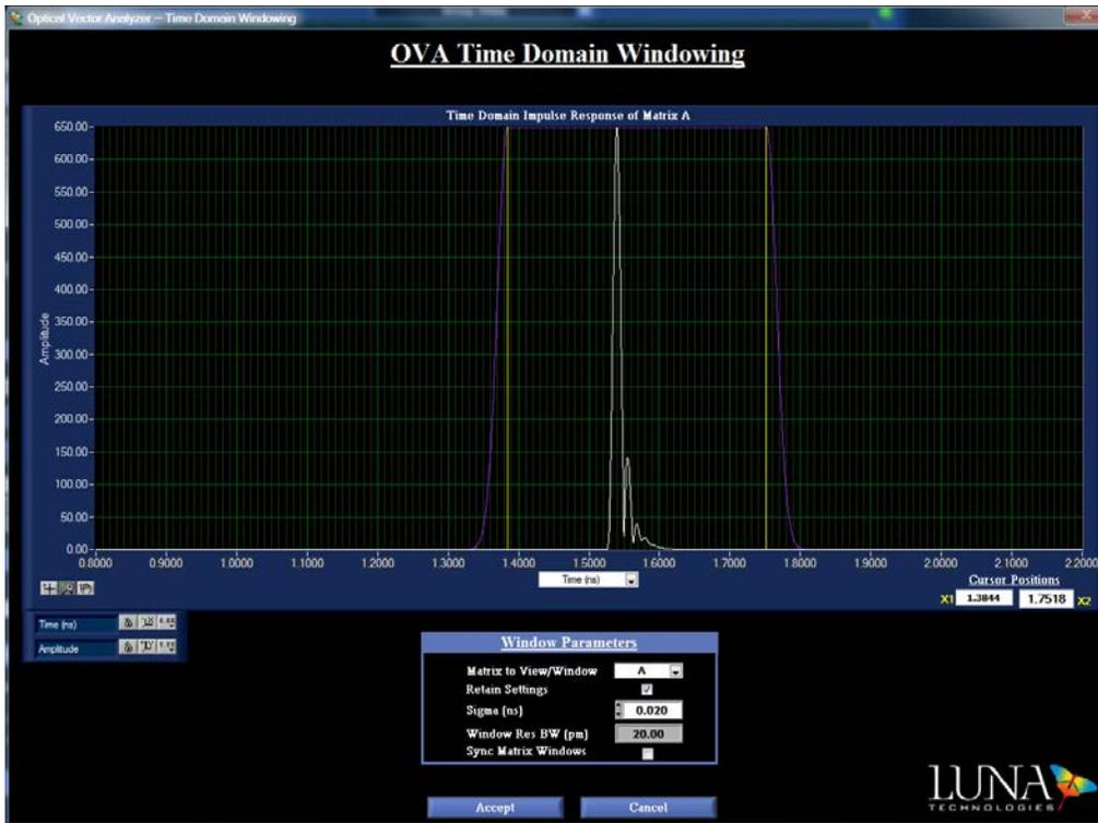
Figure 1. The time domain window and impulse response of a thin film filter.
