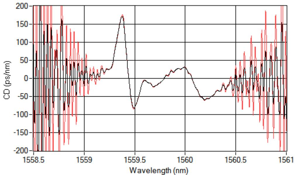
Figure 7. Chromatic Dispersion of a thin film filter measured over the -60 dB passband using an OVA 5000 with 20 pm TDRBW. (Black) CD calculated from optical phase using a 20 pm derivative step size for both the GD and CD calculations. (Red) OVA CD calculation.
