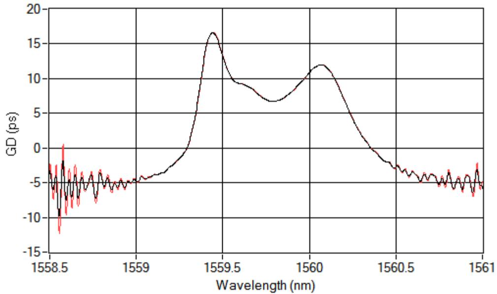
Figure 6. Group Delay of a thin film filter measured over the -60 dB passband using an OVA 5000 with 20 pm TDRBW. (Black) GD calculated from optical phase using a 20 pm derivative step size. (Red) OVA GD calculation.
