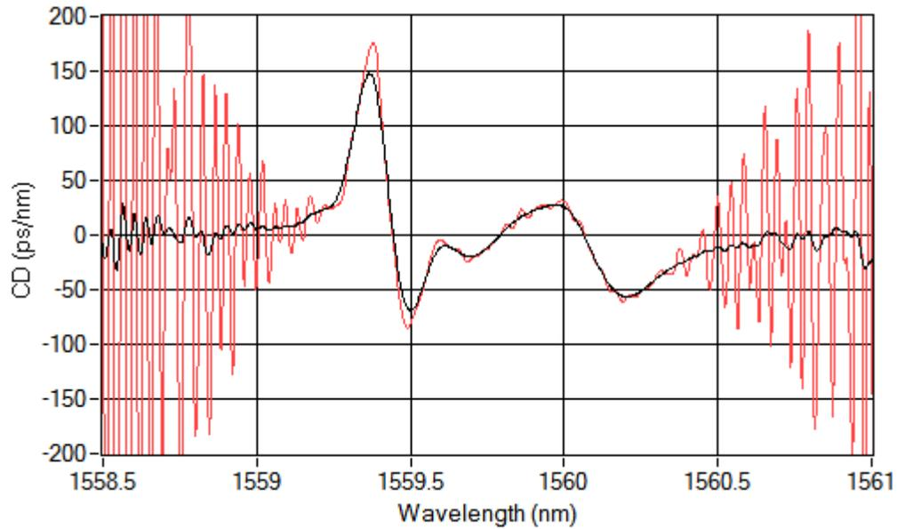
*Figure 5. Chromatic Dispersion of a thin film filter measured over the -60 dB passband using an OVA 5000 with 20 pm TDRBW. (Black) CD calculated from optical phase using a 60 pm derivative step size for both the GD and CD calculations. (Red) OVA CD calculation.*
