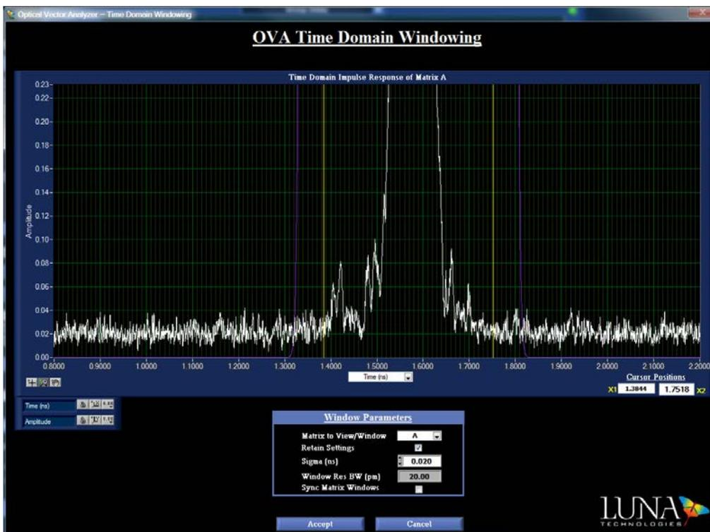
Figure 2. Vertically expanded view of Figure 1, which illustrates the impulse response is fully encompassed by a 20 pm TDRBW.
