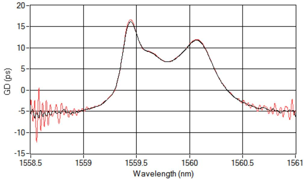
*Figure 4. Group Delay of a thin film filter measured over the -60 dB passband using an OVA 5000 with 20 pm TDRBW. (Black) GD calculated from optical phase using a 60 pm derivative step size. (Red) OVA GD calculation.*
