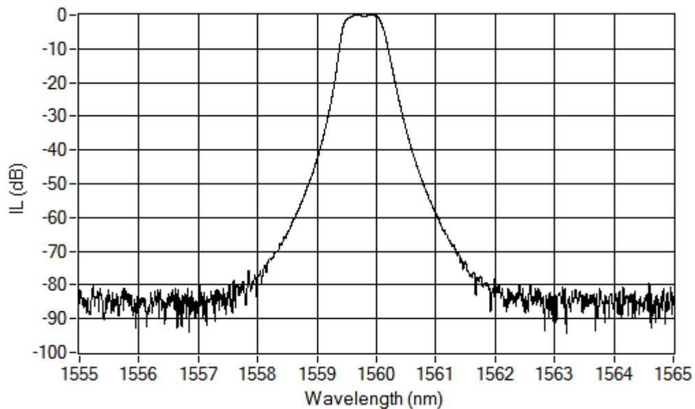
Figure 3. Insertion loss of a thin film filter measured using an OVA 5000. The TDRBW was set to 20 pm.
