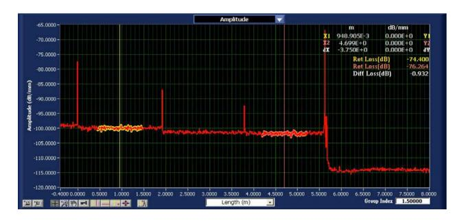
Figure 2. The OBR upper graph trace for the network depicted in Figure 1.
