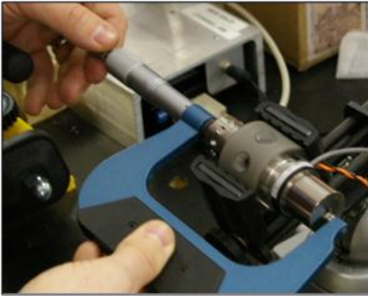
Figure 6. Empirical determination of assembly stiffness by measuring length at several preloads.
