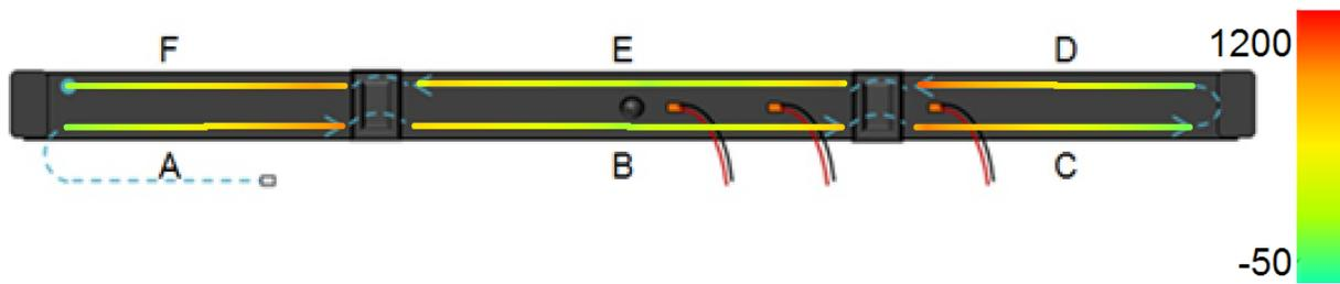
Figure 5: Map of strain along each section of the leaf spring during 135lb load case.
