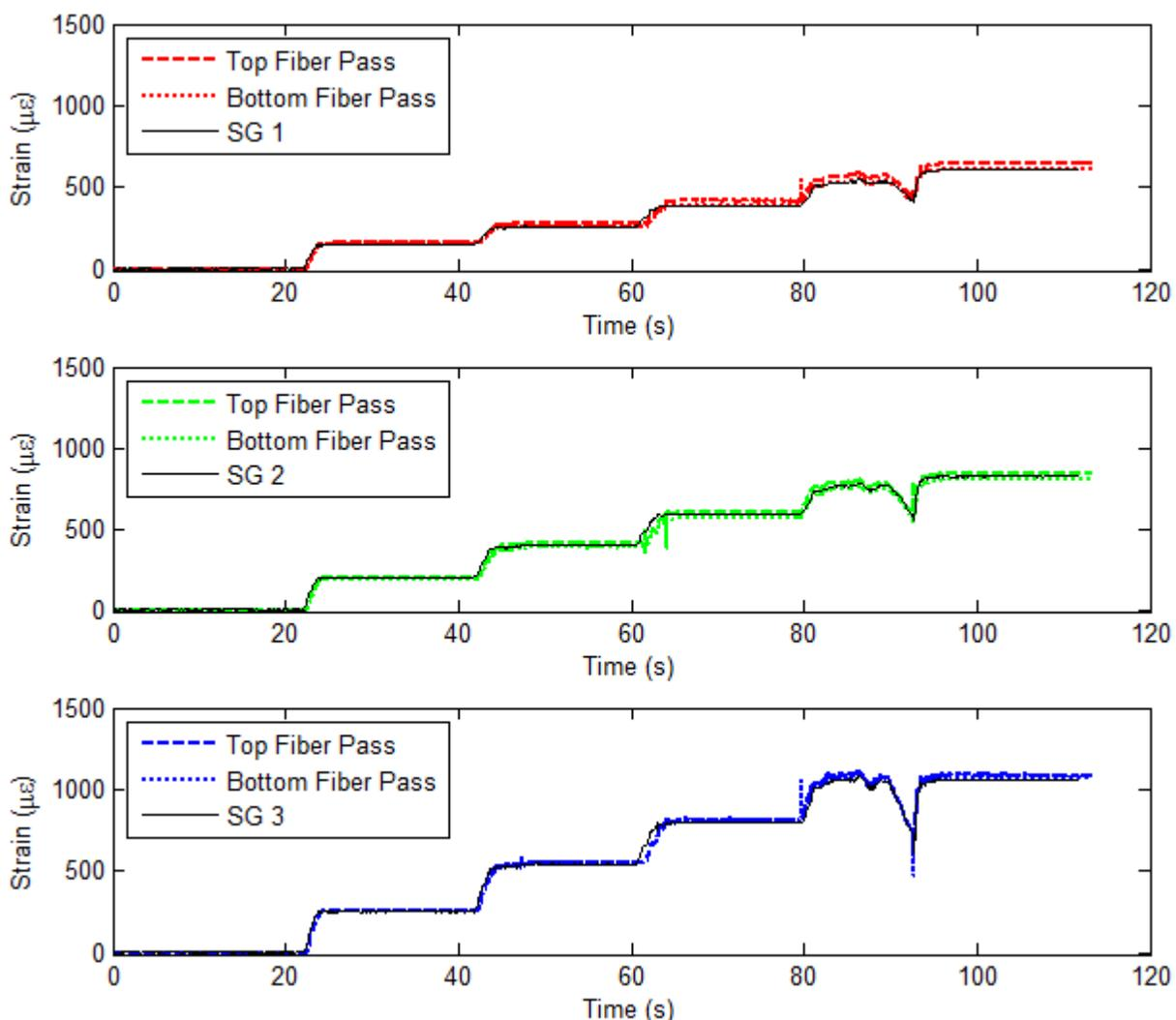
Figure 3: Single point fiber data compared to corresponding co-located foil strain gages (SG) in time. Outlier peaks are due to the physical process of adding the weights to the spring.
