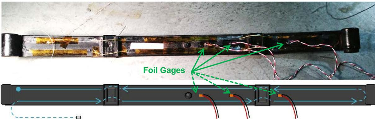
*Figure 1: Blue lines represent path of the sensing fiber, dashed lines denote regions that are not bonded. The locations of the three foil gages are also shown in orange.*
