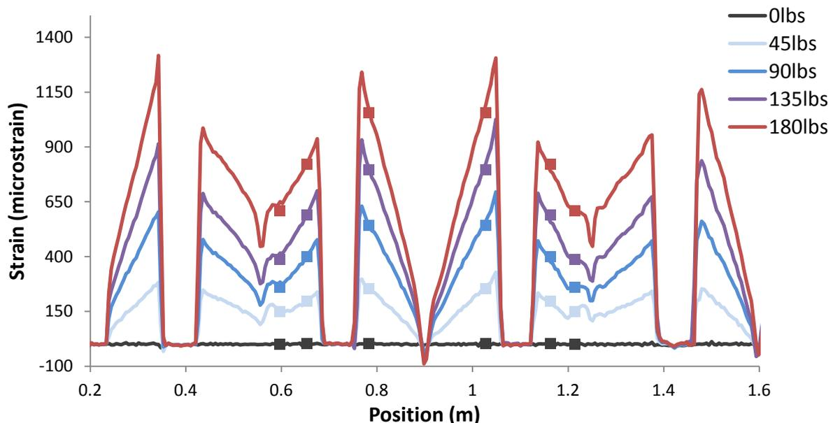
Figure 7: Strain along length of fiber for all load states with co-located strain gage measurements shown by boxes of the same color.
