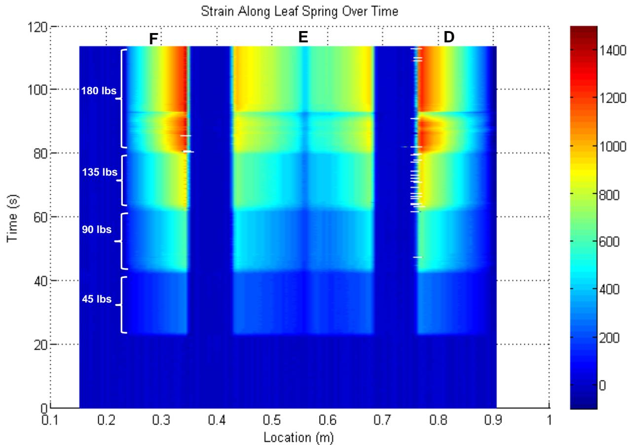
Figure 6: Strain along a single fiber pass of the leaf spring as load is increased from 0-180 lbs. Locations labeled 'F', 'E', and 'D' correspond to the same labeled locations along the leaf spring from Figure 5 above.
