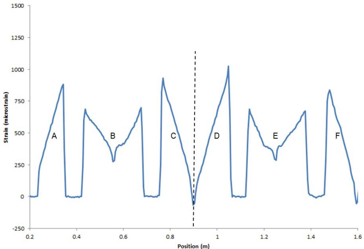
Figure 4: Strain profile along the length of the fiber at one time instance during 135lb load. The vertical dashed line shows where the fiber turns around and passes back along the length of the spring. Sections of the profile are labeled A – F, and correspond to the sections in Figure 5 below.
