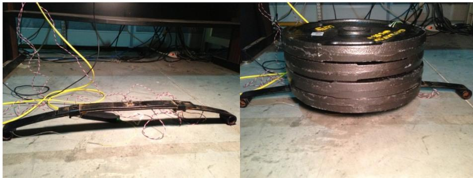
*Figure 2: Experimental setup. Leaf spring was placed on a concrete floor and loaded with four 45lb weights one by one.*
