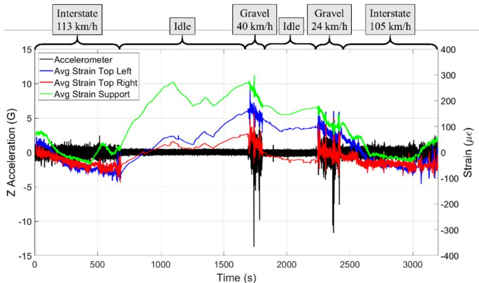
Figure 4. Accelerometer and strain measurement correlation. Z axis accelerometer data clearly shows the duration of interstate and service road conditions. The average strain for the top segments of both control arms and the support beam show corresponding times of activity. The rise in strain in between dynamic events was due to heating under the vehicle during engine idle.
