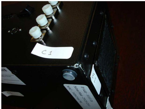
**Figure 26 – sm130 handling drop test, unpackaged equipment, typical damage, corner C1**
