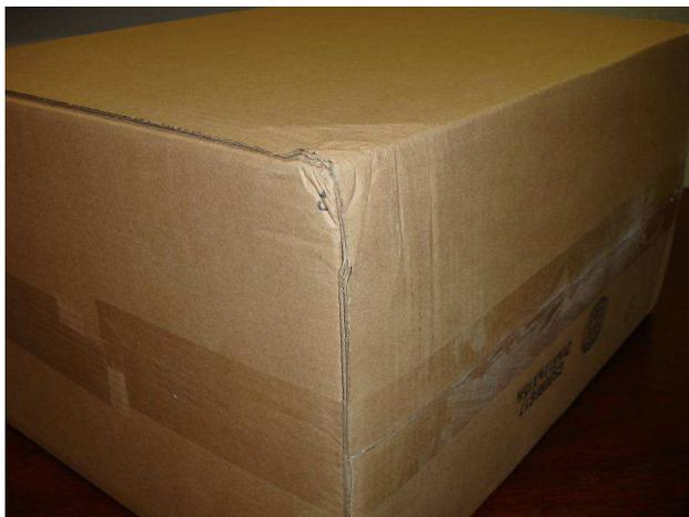
**Figure 21 - sm130 handling drop test, packaged equipment, typical damage, corner C2**
