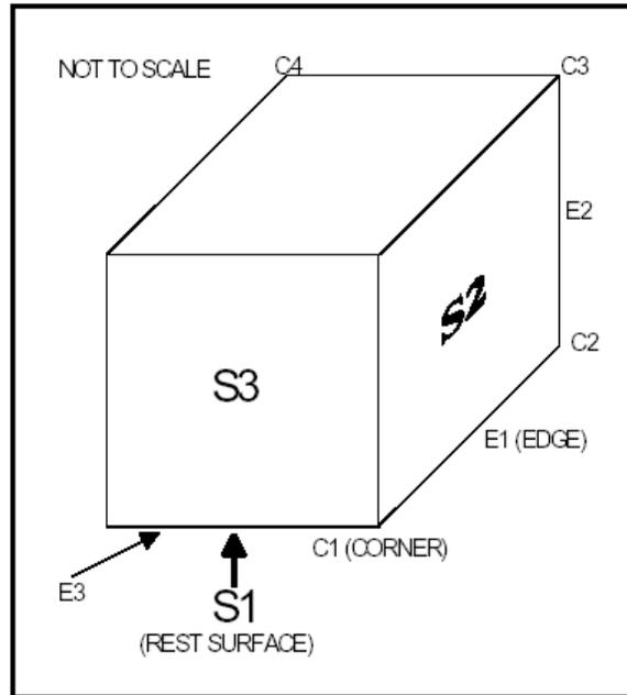
**Figure 5. Drop Surfaces for Handling Test - Packaged Container**
