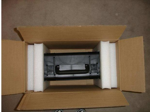
Figure 23 – sm130 handling drop test, packaged equipment, at completion of testing
