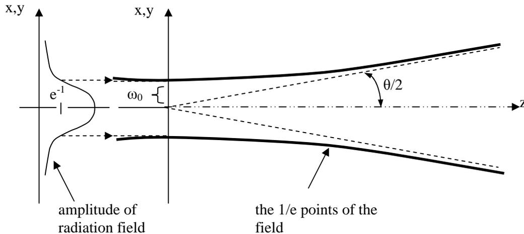
Figure 27. Beam divergence of TEM<sub>0,0</sub> mode from single mode fiber.
