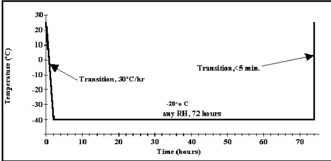
Figure 1. Low Temperature Thermal Shock
