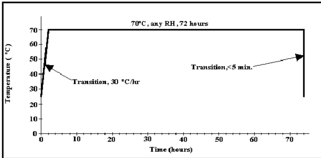
Figure 2. High Temperature Thermal Shock
