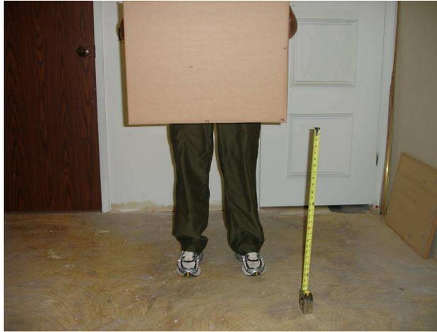
Figure 13 – sm130 handling drop test, packaged equipment, surface S1
