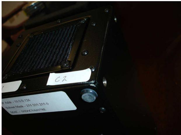
**Figure 25 – sm130 handling drop test, unpackaged equipment, typical damage, corner C2**
