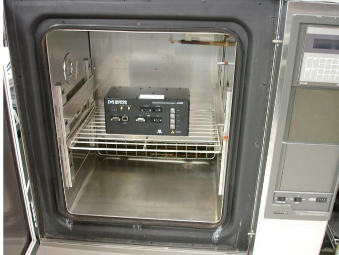
**Figure 10. EUT inside test chamber.**
