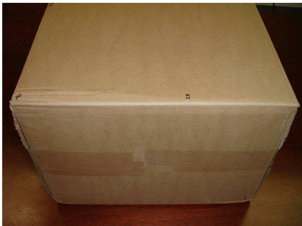
**Figure 18 - sm130 handling drop test, packaged equipment, typical damage, edge E2**
