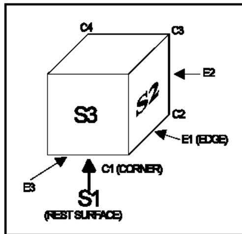
**Figure 6. Drop Surfaces for Unpackaged Equipment**
