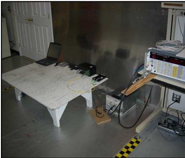
Figure 4.2.4-2: Conducted Emissions Test Setup – Side View
