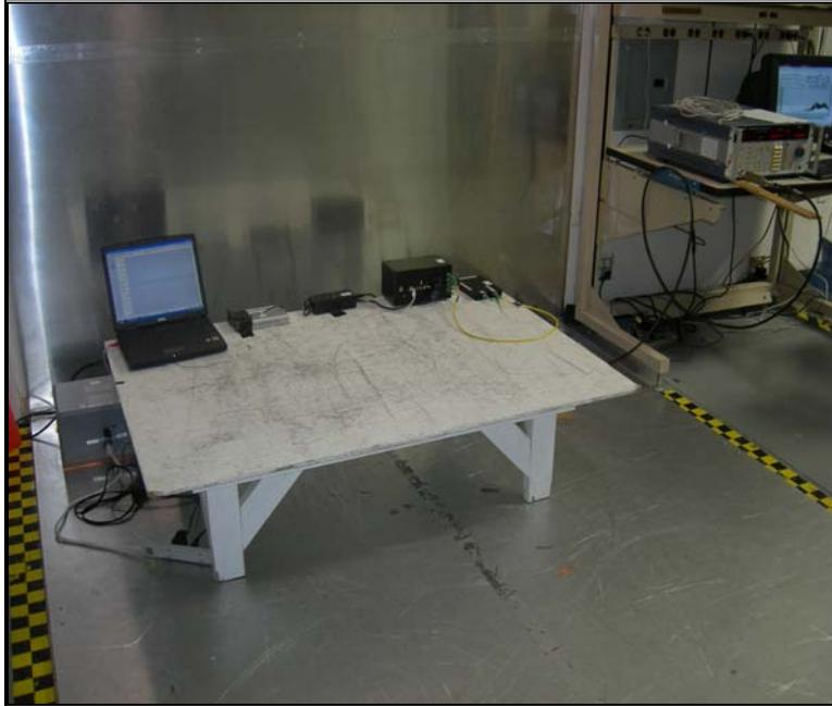
Figure 4.2.4-1: Conducted Emissions Test Setup – Front View
