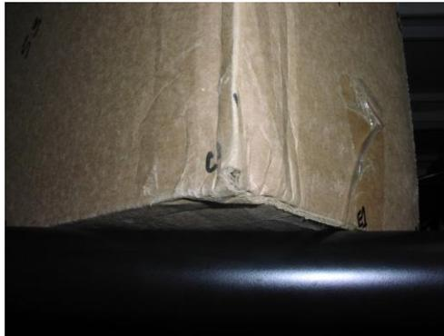
**Figures 14: Damaged corner of outer shipping container.**
