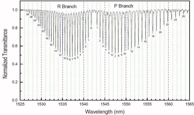
Figure 11. Plot of the HCN absorption spectrum as characterized by NIST
