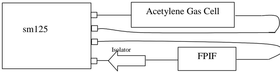
**Figure 7: Block Diagram of Test Configuration**
