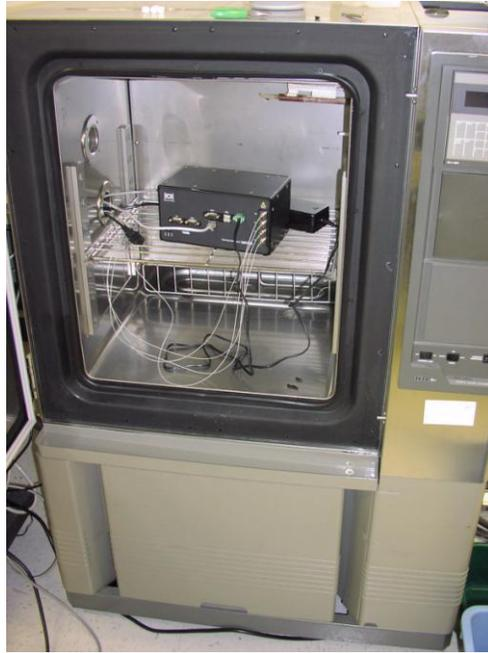
**Figure 10. EUT inside test chamber.**
