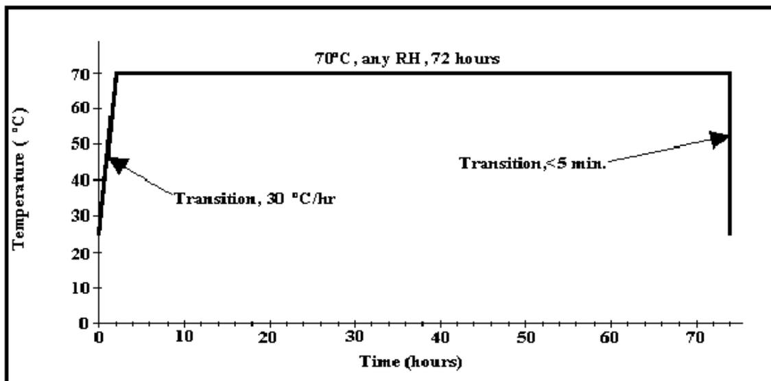
Figure 2. High Temperature Thermal Shock
