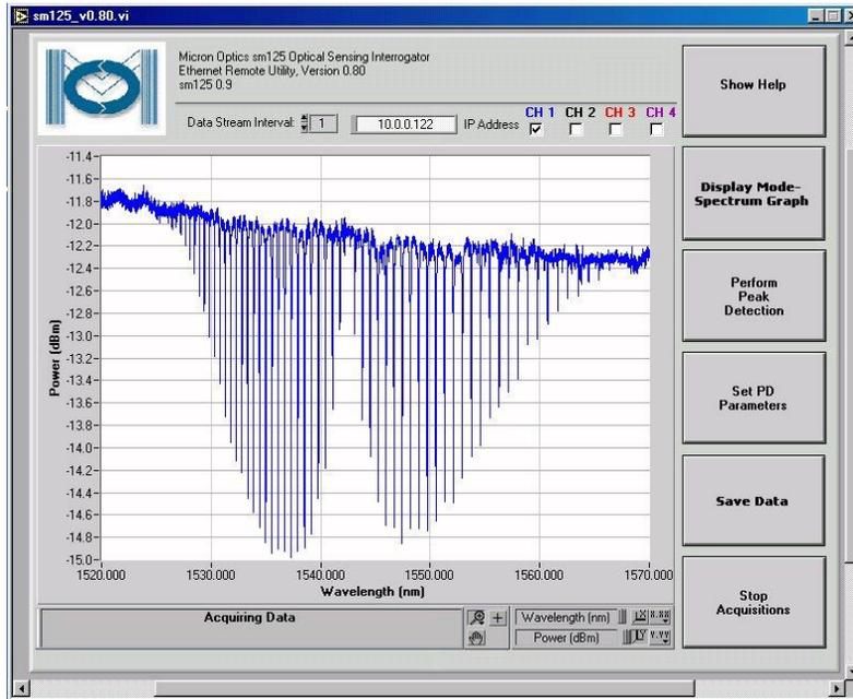
Figure 12. HCN Absorption spectrum as measured by an sm125
