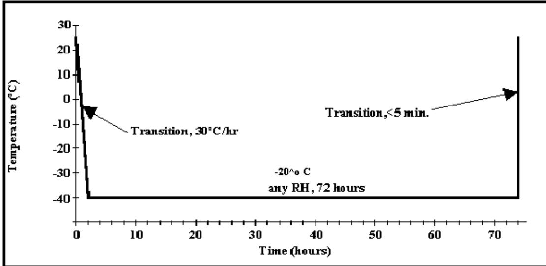
Figure 1. Low Temperature Thermal Shock
