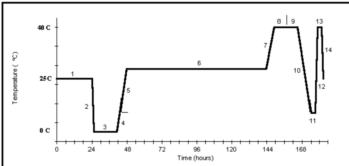
Figure 4. Operating Temperature and Humidity Test
