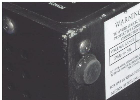
Figure 16. Slight physical damage to the corner of the sm125 after unpackaged drop testing.
