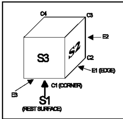
Figure 6. Drop Surfaces for Unpackaged Equipment
