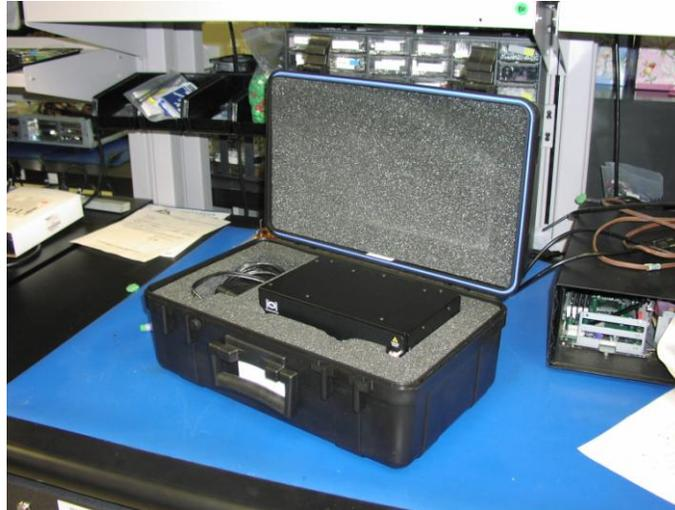
Figure15. sm125 and carrying case unaffected by drop tests.
