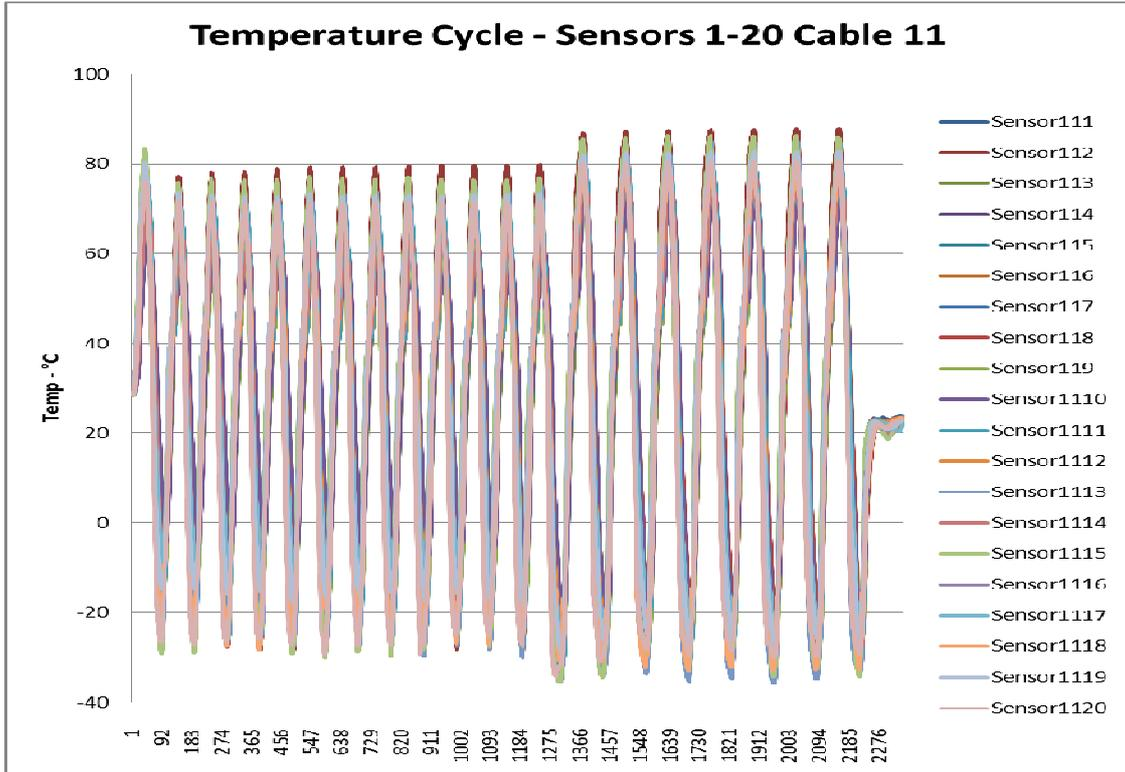
Figure 4 - Cable 11 - Sensors 1-20
