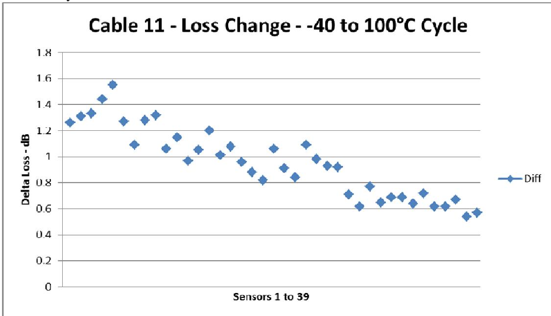
Figure 6 - Cable 11 - Sensor Loss Variation
