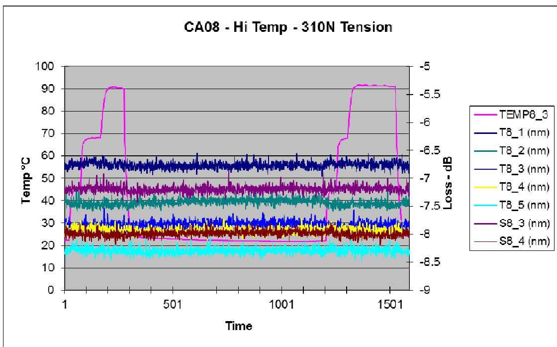
**Figure 11 - Effect on Optical Signal Loss with Temperature Variation**
