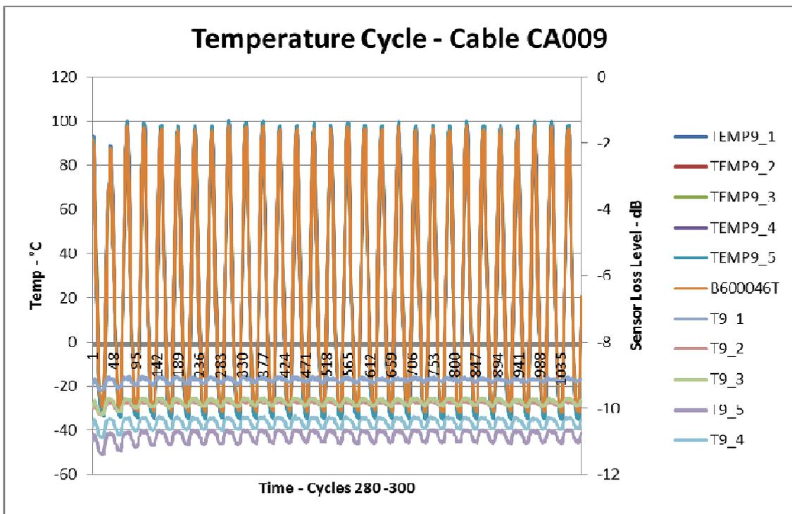
Figure 2 - Graph - Sensor Temperature and Loss
