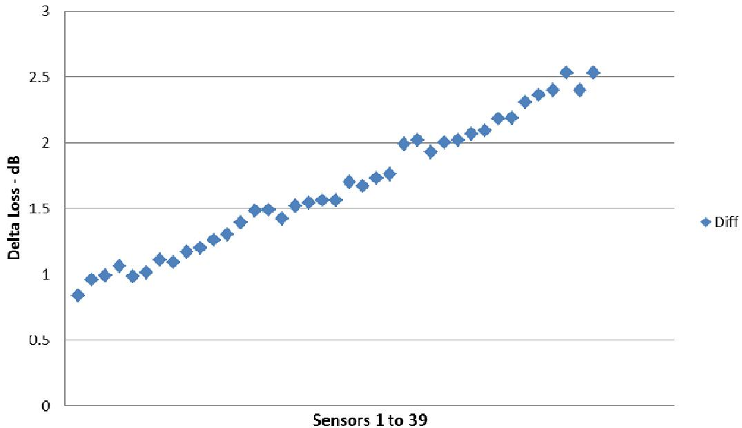
**Figure 9 - Cable 12 – Effect of Temperature on Cumulative Optical Loss at each Sensor Point**
