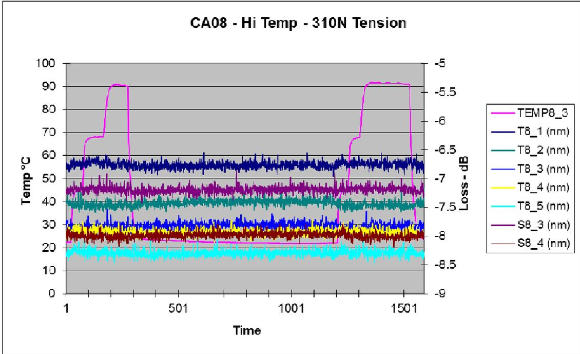
Figure 11 - Effect on Optical Signal Loss with Temperature Variation
