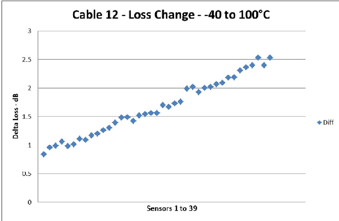
Figure 9 - Cable 12 – Effect of Temperature on Cumulative Optical Loss at each Sensor Point
