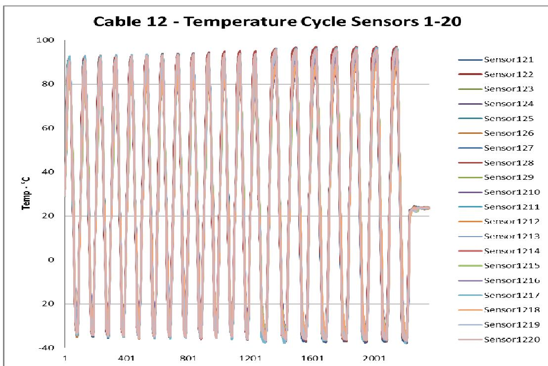
Figure 7 - Cable 12 - Sensors 1-20
