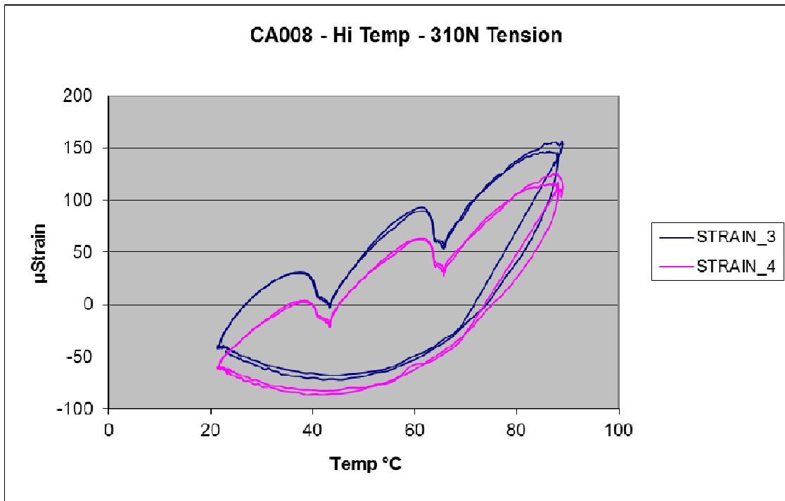
**Figure 10- Cable CA008 – Effect of Temperature on Fiber Strain**
