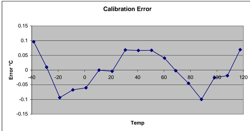
**Figure 3 – Typical Error from 3<sup>rd</sup> order Polynomial Curve Fit**
