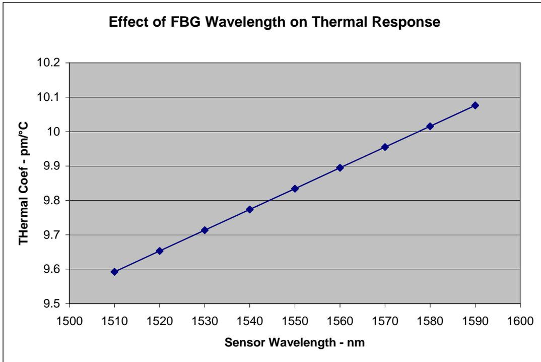
Figure 2 – Effect of Wavelength on Thermal Response
