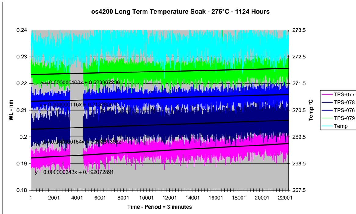
**Figure 4 – Raw Data from Long Term Temperature Soak**
