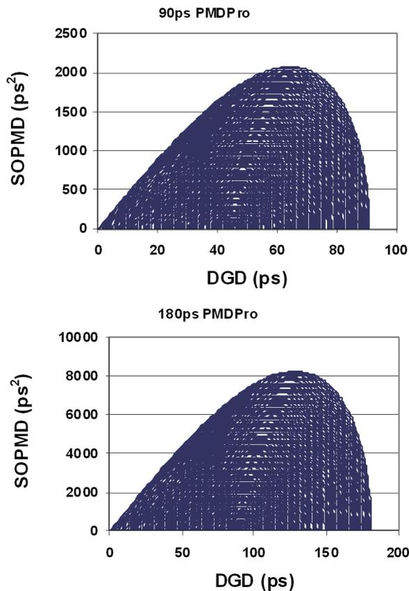
Figure 7 DGD and wavelength independent SOPMD range
