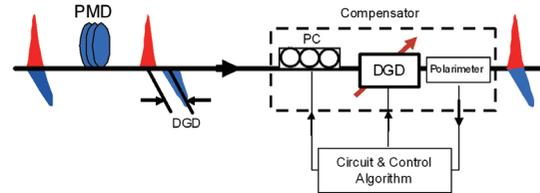
Figure 2 Optical PMD compensation. The DOP measured by the polarimeter is used as PMD effect indicator.
