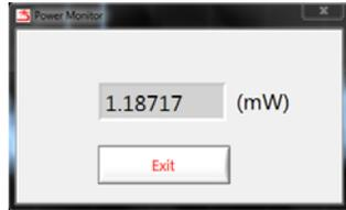
Check that the optical power is at an appropriate level. Power  $\sim 1\text{mW}$  or so usually works well. If the power is too high or too low, change the attenuator setting (range 0 to 30 dB) and check the power again.
