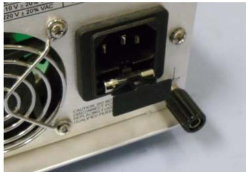
**Figure 5 Fuse compartment**
