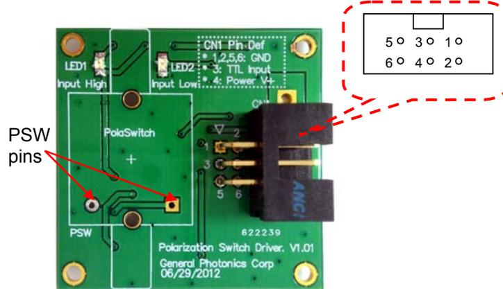
**Figure 11 PSW driver board dimensions and pinout**
