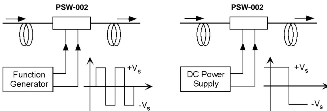
**Figure 9 Examples of basic driver setups. A function generator can be used to drive the PSW for periodic switching, while a DC power supply may be sufficient for occasional switching. Note that this diagram shows only switching voltages. Once the device has switched state, the voltage can be lowered to the latching voltage to maintain the output state.**
