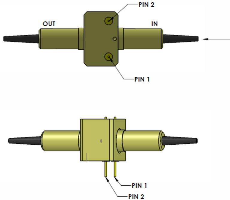
**Figure 6 PSW-002 pinout**
