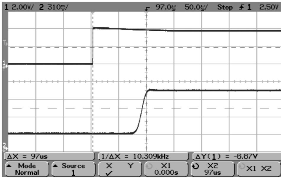
Figure 7 Switching speed of PSW-002 under a -2 to +2V voltage step
