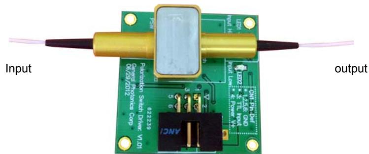
Figure 10 PSW-002 on driver board
