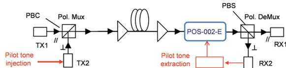
Scheme 1: Pilot tone detection. A low frequency pilot tone around 100 kHz is injected at one of the transmitters. At the receiving end, a pilot tone extraction circuit can be used to detect the strength of the pilot tone and convert it into a 0-5V feedback signal for the POS-002-E. The detected pilot tone will be maximized when the two polarization channels are properly separated. The polarization tracker then automatically maximizes the feedback signal to separate the two polarization channels.
