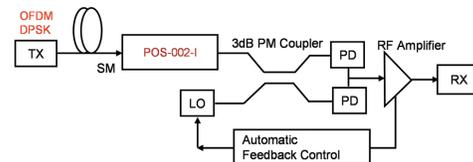
In a coherent detection system, the states of polarization of the signal and local oscillator must be the same in order to maximize signal to noise ratio. A POS-002-I can be used to stabilize the SOP of the signal after it propagates through the transmission fiber. The SOP of the output of the polarization tracker is linear and aligned with the slow axis of the PM fiber pigtail and will beat with the local oscillator.
