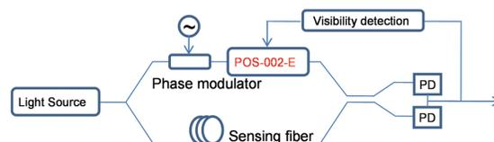
In an interferometric sensor system, the detection sensitivity is directly related to the SOPs of the two interfering signals. A POS-002-E can be used to obtain the maximum detection sensitivity. In this application, the visibility of the sensor can be monitored with a phase modulator and can be converted into an analog signal of 0-5 volts to be fed back to the POS-002-E. The polarization tracker then automatically maximizes the visibility for stable, optimized detection sensitivity.
