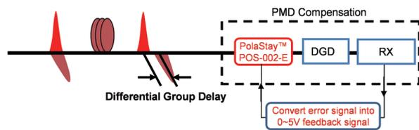
Scheme 2: Using the receiver to obtain the feedback signal. In this scheme, the error signal indicating the PMD effect can be a clock signal from the receiver's photodetector or a BER detected before FEC inside the receiver. The user converts the error signal into an analog signal between 0-5 volts and feeds it back to the POS-002-E. The polarization tracker then either maximizes or minimizes the error signal to achieve PMD compensation.
