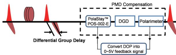
Scheme 1: Using a polarimeter to obtain feedback signal. In this scheme, a polarimeter is used to detect the degree of polarization (DOP) of the signal to indicate the PMD effect on the signal. The DOP will be maximized when the PMD is properly compensated. The user constructs a simple circuit to convert DOP into an analog signal between 0-5V and feeds this signal back to the POS-002-E. The polarization tracker then automatically maximizes DOP to achieve PMD compensation.
