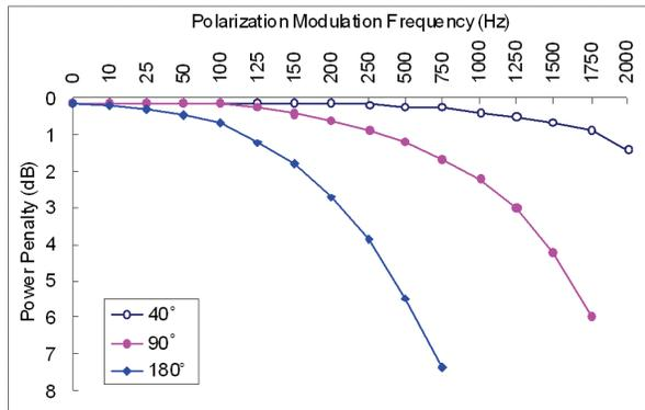
Figure 3. POS-002-I tracking of sinusoidal polarization modulation.
