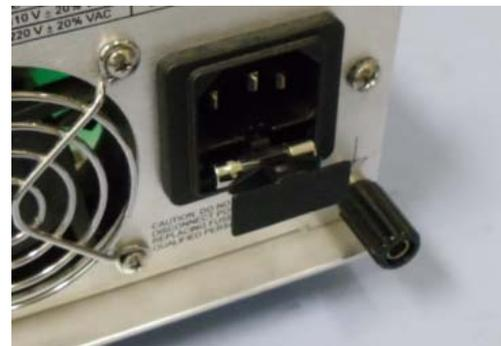
**Figure 6 Fuse compartment**
