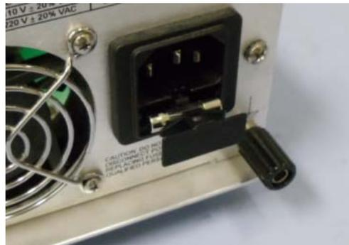
**Figure 6 Fuse compartment**
