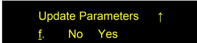
With the cursor on the index number (a-f), use the wheel to move between static IP setup parameter options.
