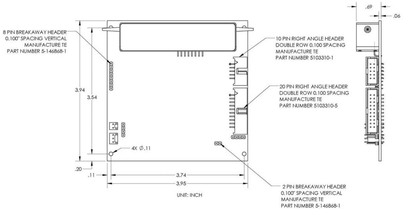
**Figure 4 Dimensions of MPD-001/PCD-M02**
