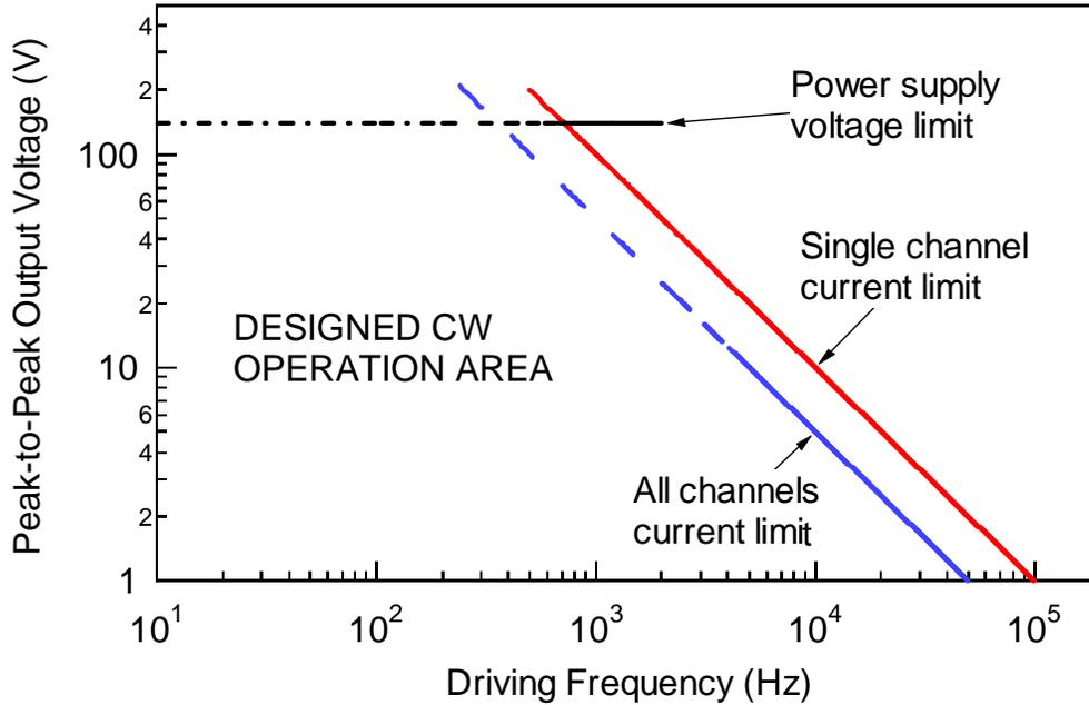
**Figure 7 Current limit and power supply constraints on the peak-to-peak output voltage and driving frequency. The black horizontal line is the power supply high voltage limit. The red solid line is the single channel operation current limit. The blue broken line is the total current supply limit when all 4 channels are driven by a single sine frequency.**
