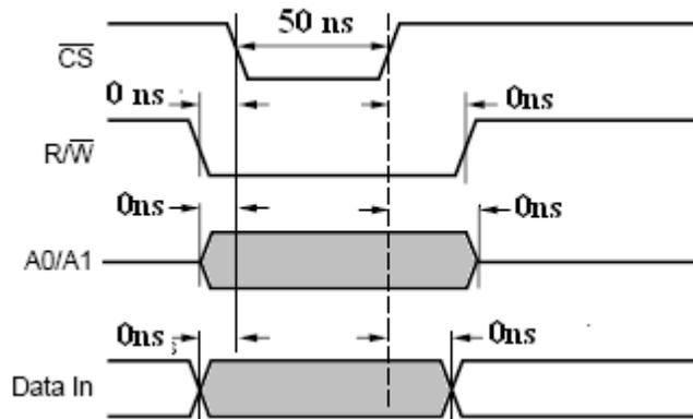
**Figure 6 Timing diagram to write data to the MPD-001/PCD-M02**
