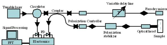
Fig. 2 Scanning Laser Based Frequency Domain OCT (FD-OCT)
