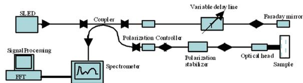
Fig. 3 Spectrometer based Frequency Domain Optical Coherence Tomography (FD-OCT)
