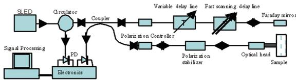
Fig. 1 Time Domain Optical Coherence Tomography (TD-OCT)
