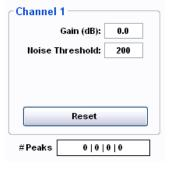
For x30 interrogator cores, peak detection is performed in channel hardware and during the actual laser scan. As such, the peak detection parameters are common among all of the sub-channels that make up a channel group, as
