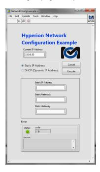
To change the network Settings on the module, the user would enter the target HYPERION's current IP address into the **Current IP Address** control and click run. Then by making selections among **Static IP Address/DHCP (Dynamic IP Address)**, setting the pertinent specific parameters, and clicking the **Execute** button on the UI, the HYPERION Instrument will be updated accordingly. The updated settings will then be reflected on the panel mounted LCD screen of the unit.
