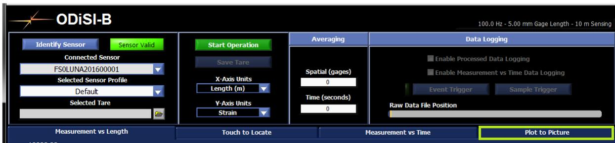
Figure 3-23 Plot to Picture tab location
