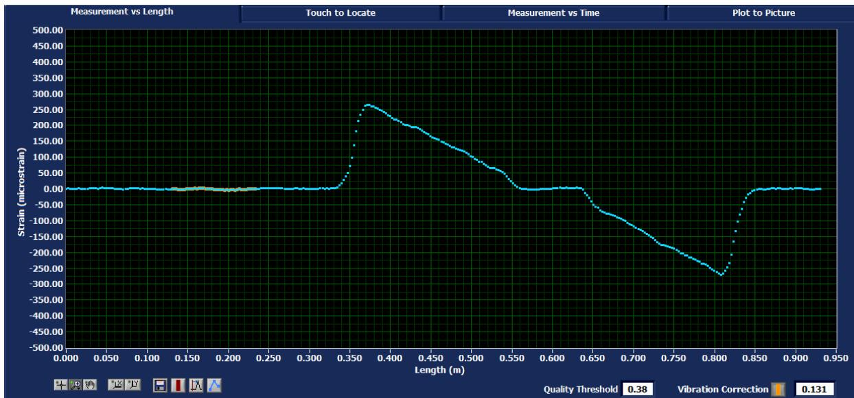
Figure 4-22 Measurement vs. Length tab of the ODiSI-B interface
