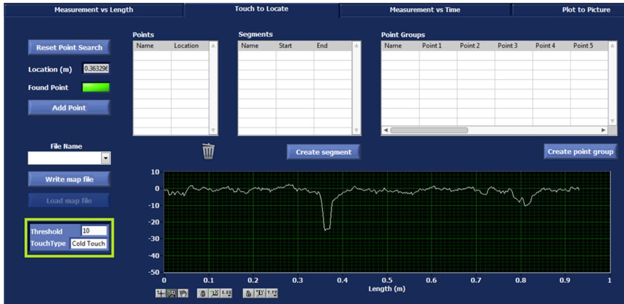
Figure 3-12 Threshold and Touch Type control locations
