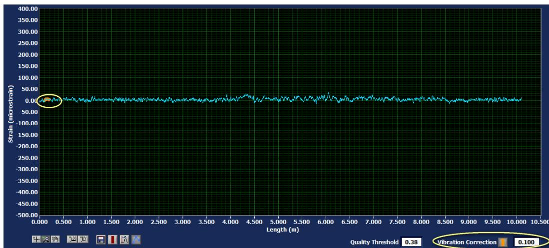
Figure 3-9 Vibration Correction trace (orange highlight in graph) and Vibration Correction location control
