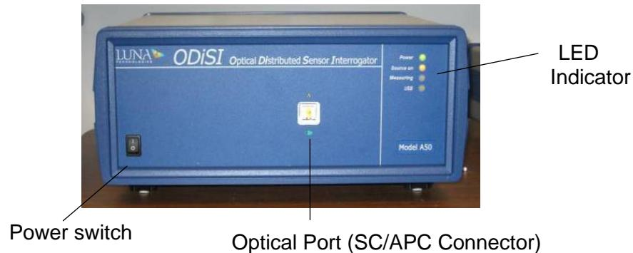
Four LEDs indicate the state of the instrument:
