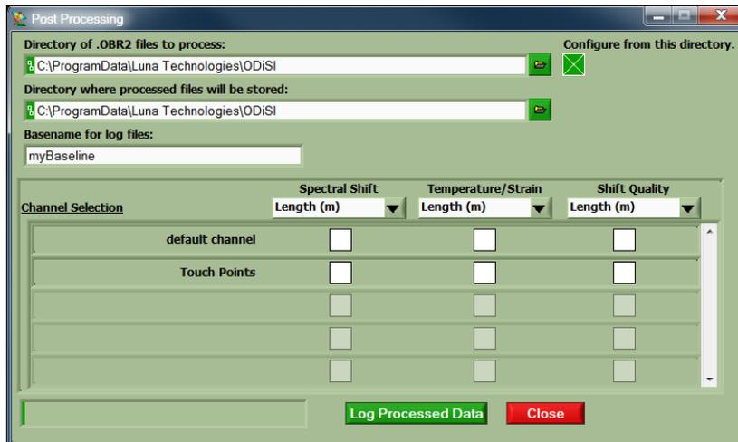
3-10 The Post Processing Window. Use to convert logged data files into text files.
