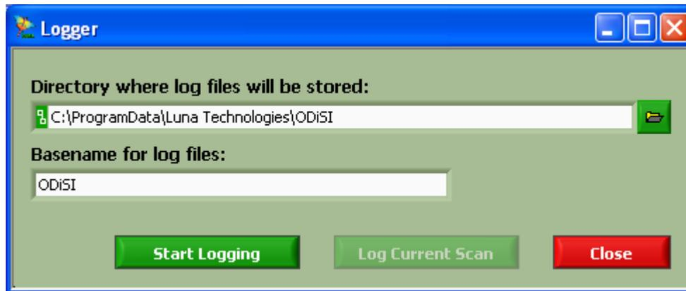
Figure 3- 8 The Data Logger Window. Use to set where and if raw measurement data will be logged, or saved.
