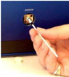
*Figure 9-1. Open the protective cover. Gently insert supplied mini swab, rotate in one direction, then remove.*
