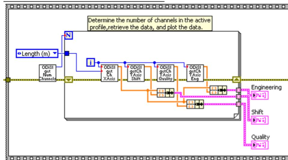
Figure 5-9 Plot measurement results
