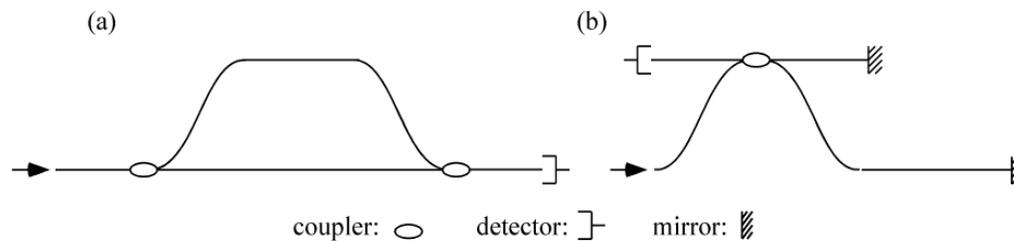
Figure 6- 1 Two basic types of fiber interferometers:
