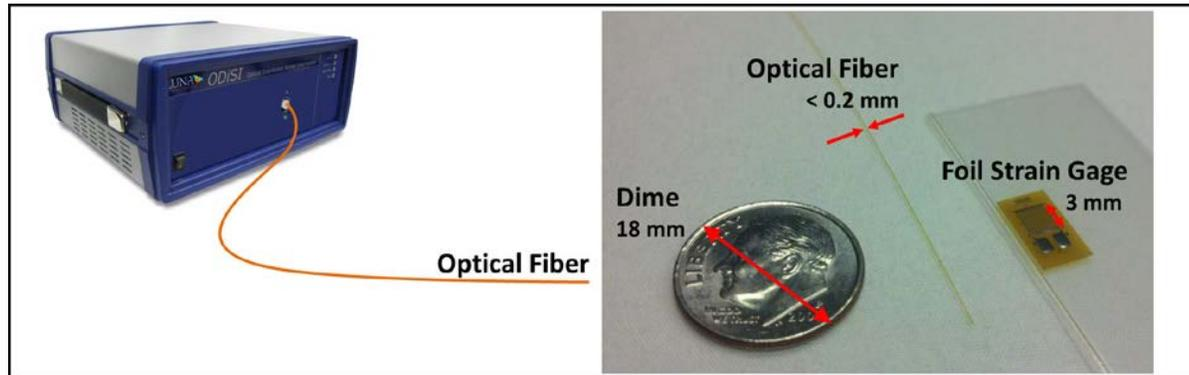
Figure 1-1. Figure 1-1 ODiSI sensor fiber is much thinner and longer than traditional foil strain gauges.
