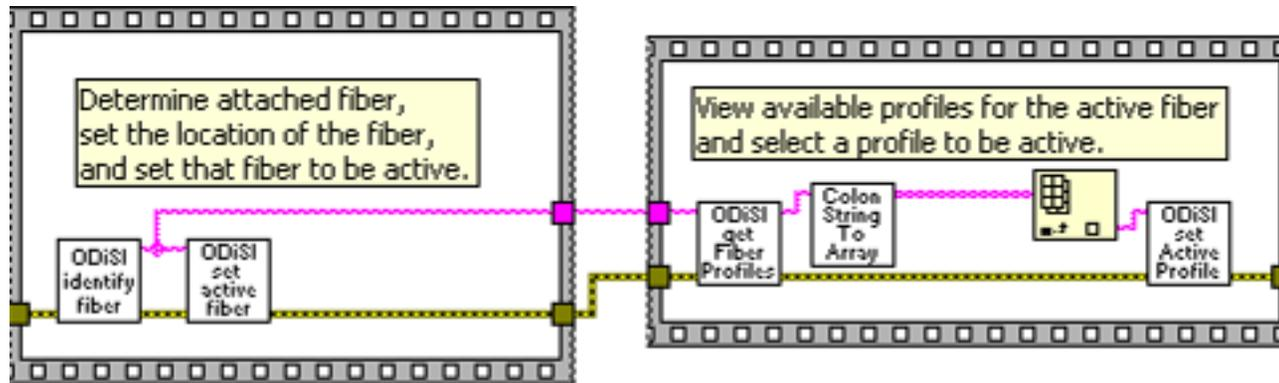
Figure 5-3 Identify the attached fiber, set active fiber, and set active profile.
