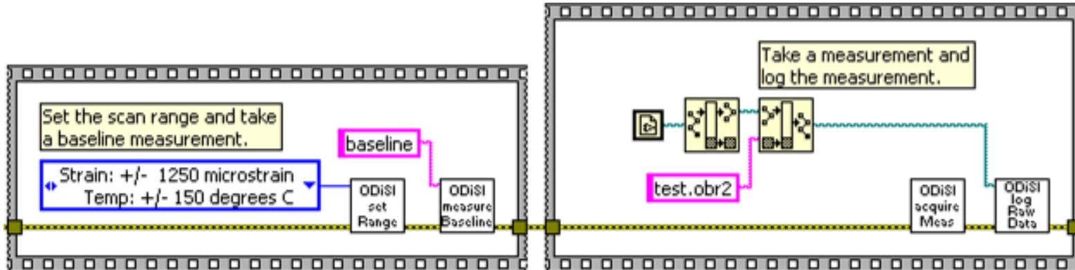
Figure 5-4 Set scan range, take a baseline, acquire a measurement, and log the measurement.
