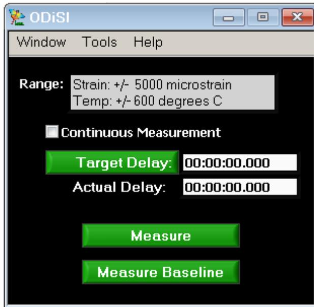
*Figure 1-3. Control software initial window. The window will be inactive when the software starts. It will become active when the instrument completes its self test.*
