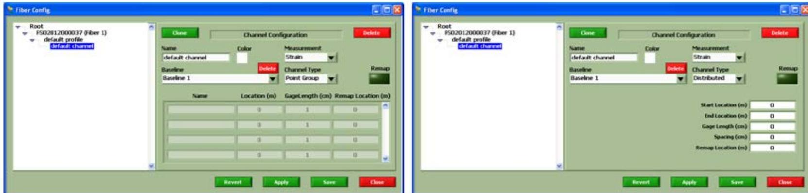
3-6 Channel Configuration Display. The display appearance is changed by selecting Point Group or Distributed Channel Type.
