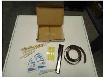
Getting started kit includes: 1 meter temperature sensing fiber, 1 meter strain&temperature sensing fiber, and 2 meters of fiber to practice attaching fiber to a structure.
