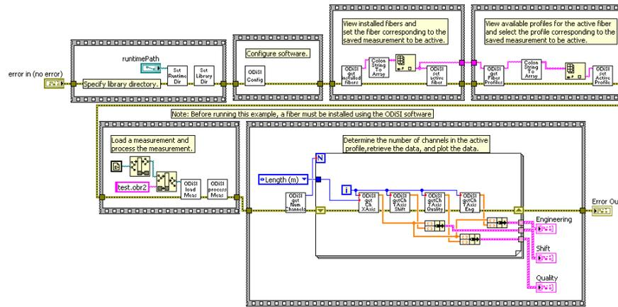
Figure 5-5 SDK Load Plot.vi
