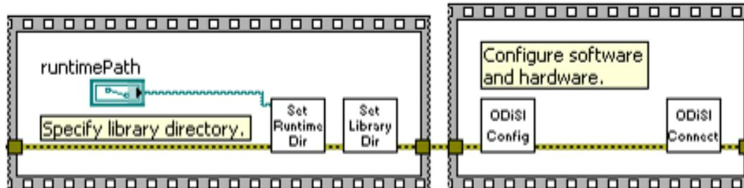
Figure 5-2 Set runtime directory, configure software, and connect to the system.
