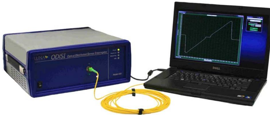
Figure 1-2 ODiSI measurement system. The ODiSI measures strain and temperature at user specified locations along the fiber. Data is presented graphically, providing the user with unprecedented data density and resolution.
