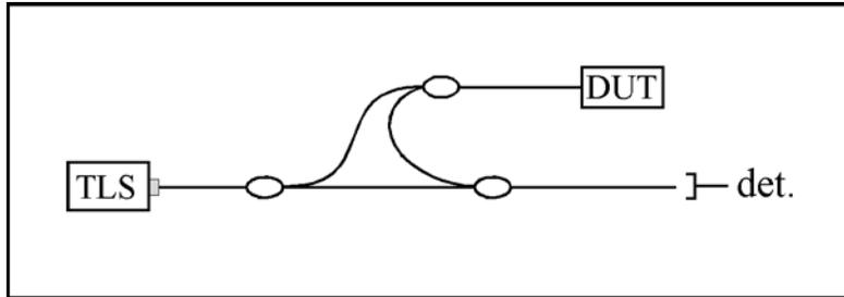
Figure 6-2 ODiSI optical network
