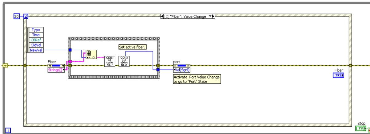
Figure 3: "Fiber" State of event structure
