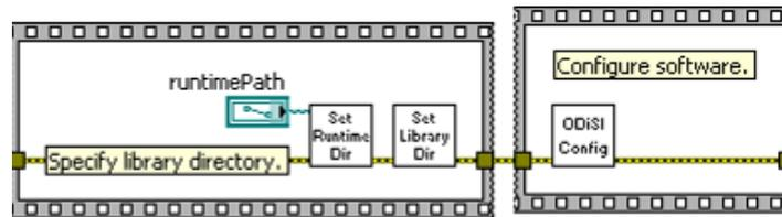
Figure 5-6 Set runtime directory, configure software, and connect to the system.
