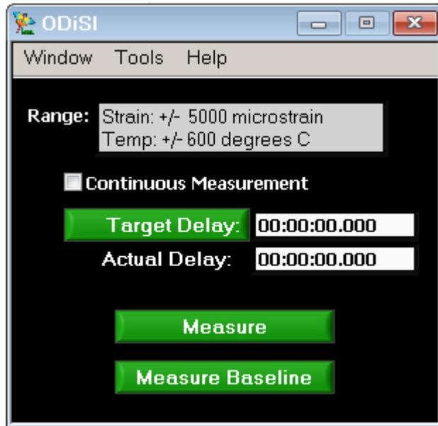
Figure 3- 1 ODiSI Control window is the main user interface
