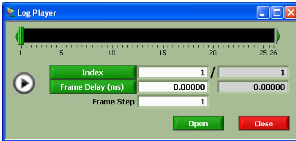
Figure 3- 9 The Log Player Window. Use to replay data that was previously logged.
