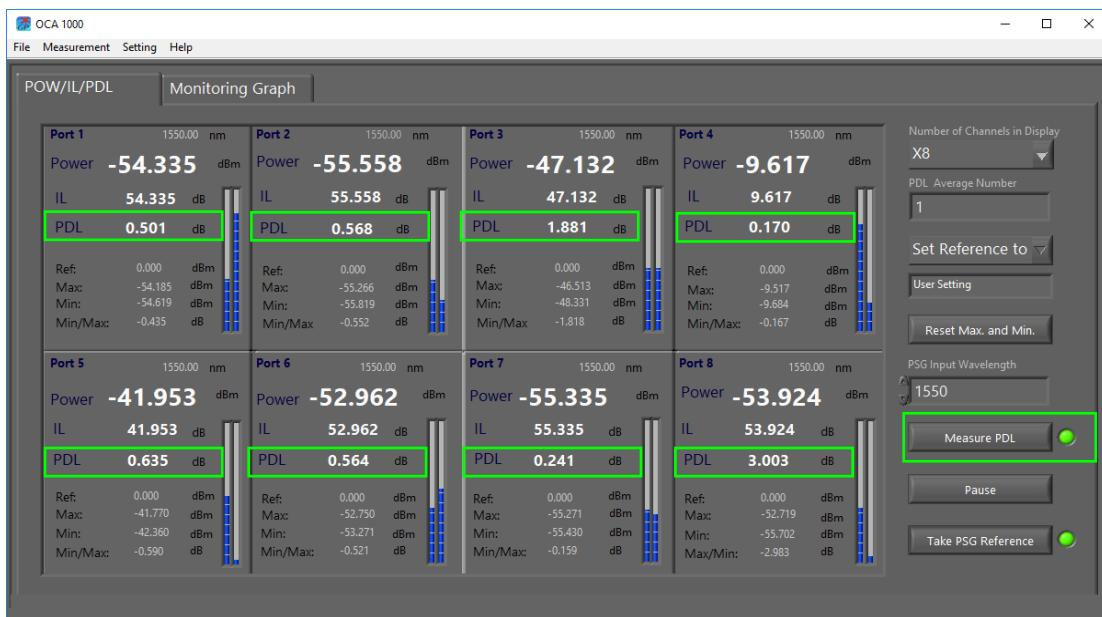
**Figure 13 PDL measurement result.**
