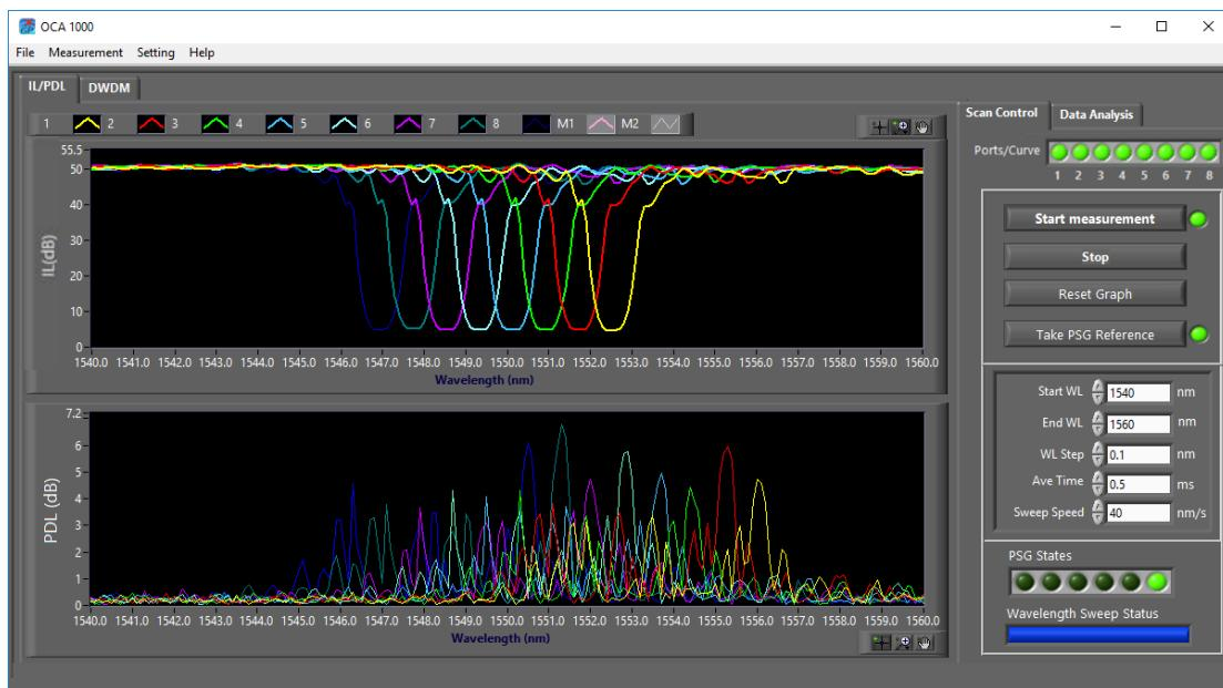
**Figure 14 IL/PDL vs. wavelength measurement of an 8-channel C-band AWG measured with a 1540-1560nm wavelength sweep**
