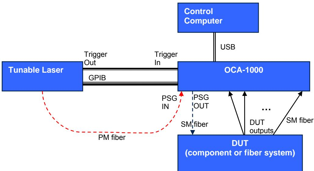
**Figure 6 Power/IL measurement setup.**
