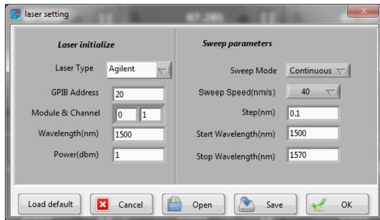
Make sure that the communication setup is correct and that the power level is within the range of the laser used. Sweep settings can be set either from this screen or directly from the measurement screen.
