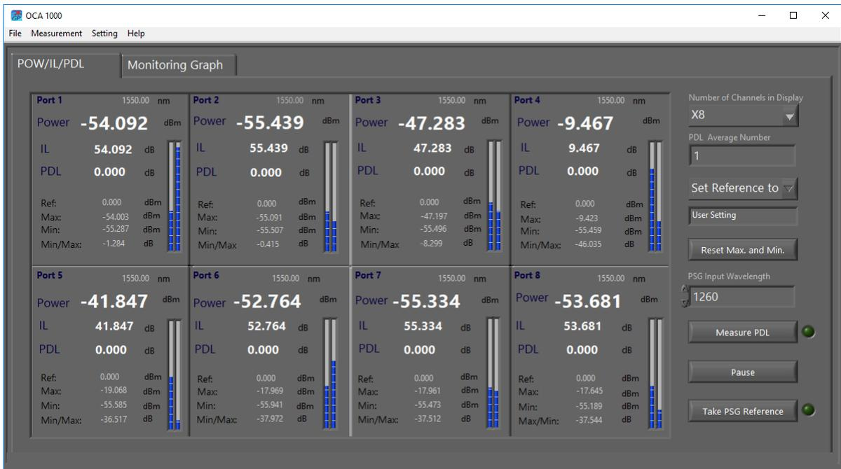
Figure 7 POW/IL/PDL measurement screen, 8-channel view. DUT is an AWG.
