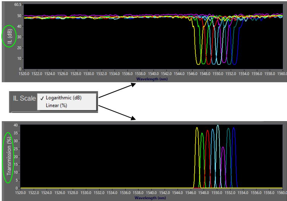
Figure 17 Wavelength scan IL plot y-scale options
