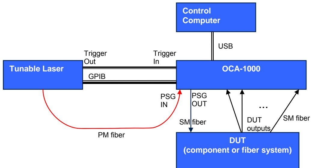
**Figure 4** Setup diagram for PDL/IL measurement
