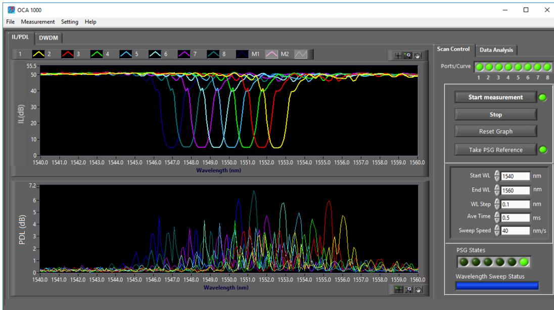
**Figure 14 IL/PDL vs. wavelength measurement of an 8-channel C-band AWG measured with a 1540-1560nm wavelength sweep**
