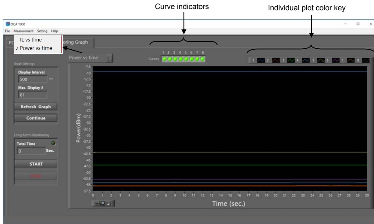
**Figure 10 Monitoring graph display for power measurement**
