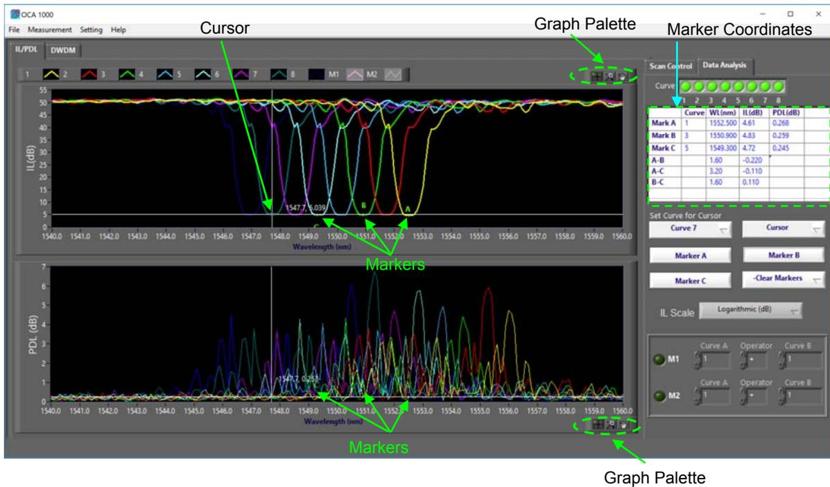
Figure 15 Wavelength scan IL/PDL graph example (DUT is an 8-channel C-band AWG) with 1 cursor and 3 markers on screen
