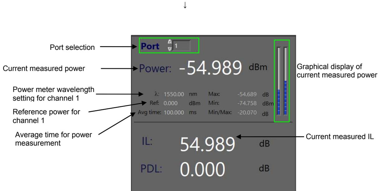
**Figure 9 Closeup of a data display panel from the 2-channel display**
