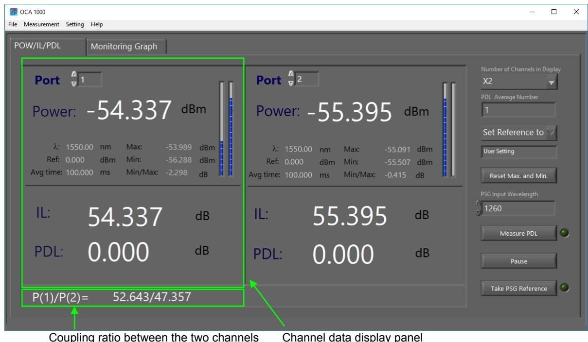
**Figure 8 POW/IL/PDL screen, 2-channel view.**
