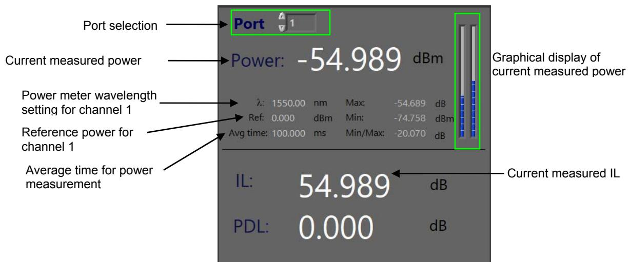
**Figure 9 Closeup of a data display panel from the 2-channel display**
