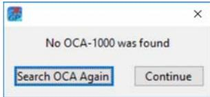
If this message appears while an OCA-1000 is connected to the computer, check the USB connection. Make sure that the OCA-1000 is connected to the USB 2.0 port of the computer and is powered on. The connection between the OCA-1000 and the control computer can be confirmed from Device Manager. Open Device Manager on the control computer and check the ports. There should be one standard USB Serial Port under "Ports (COM & LPT)".
