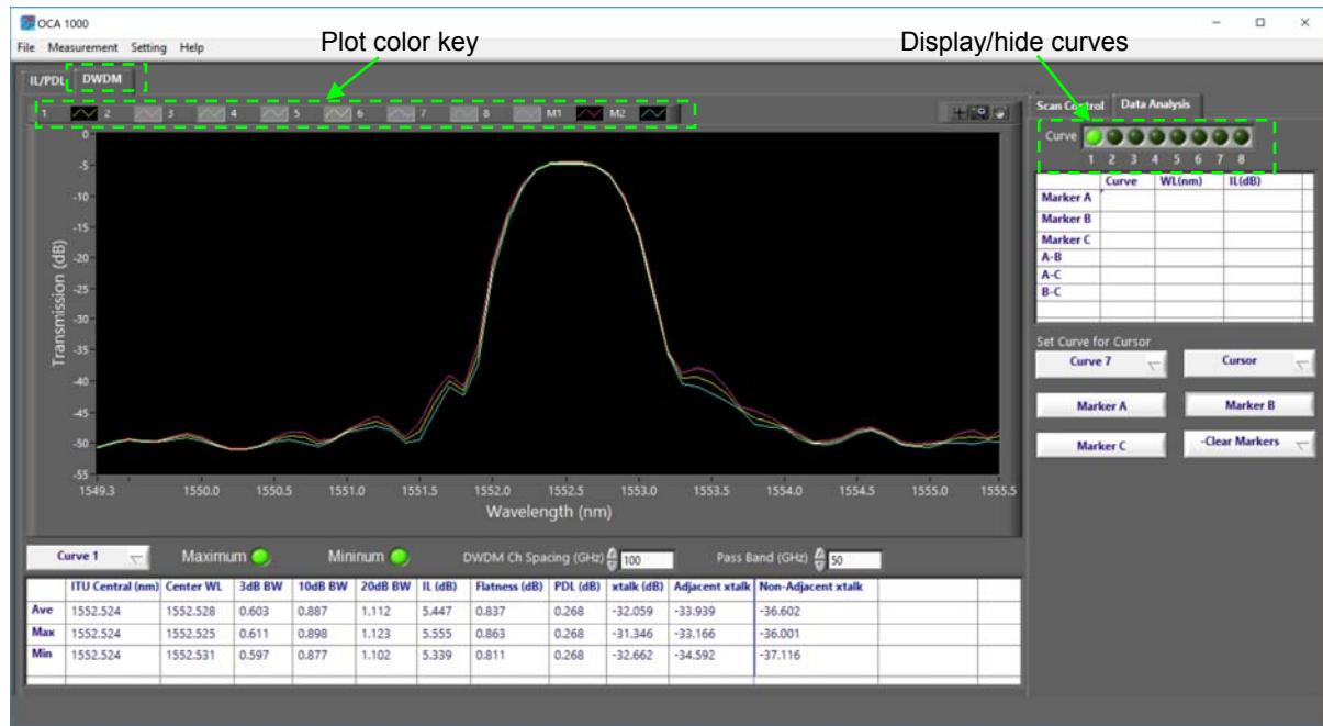
The plot shows the transmission (in dB) vs. wavelength for all displayed channels. Curves can be displayed or hidden by clicking the corresponding indicators in the control pane on the right of the screen.
