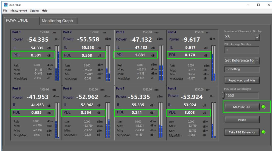
Figure 13 PDL measurement result.
