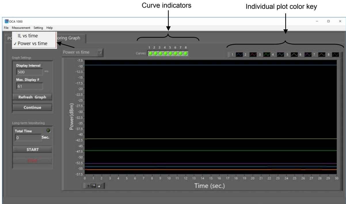
**Figure 10 Monitoring graph display for power measurement
