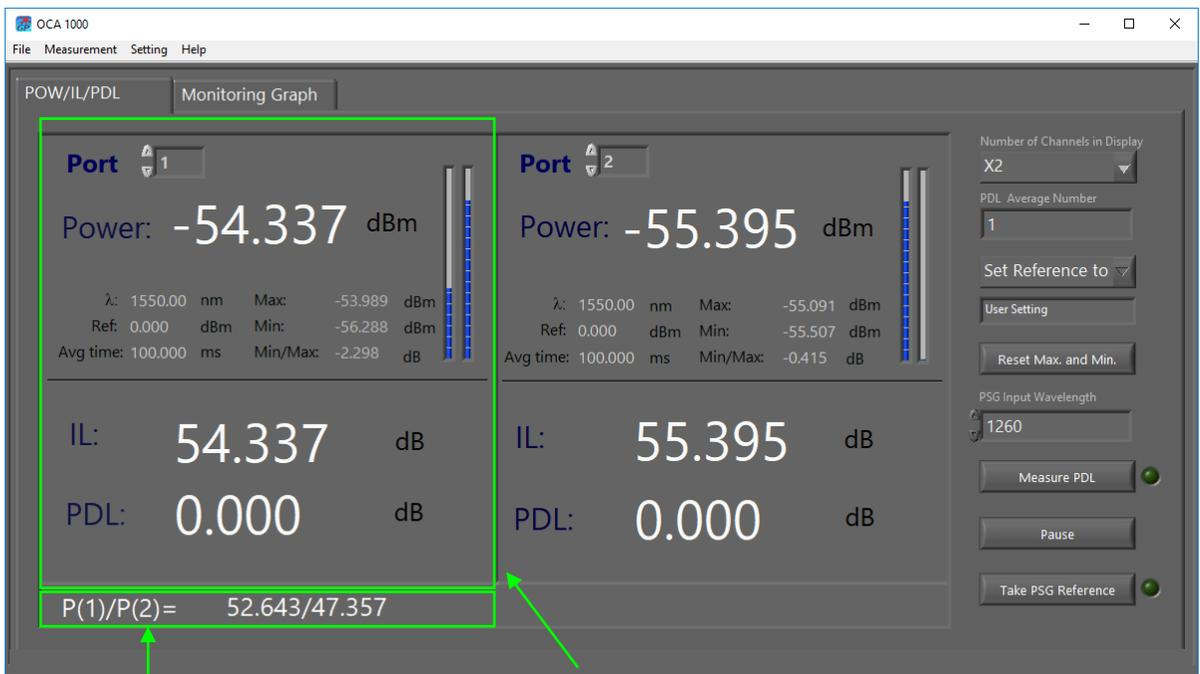
Coupling ratio between the two channels      Channel data display panel
