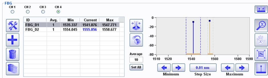
In the image above, the FBG “FBG\_D1” has been selected, and its image has been highlighted on the graph in blue to aid with visual association. Also note that the FBG bin limits for all other FBG entries have been grayed out, further highlighting the selected FBG and its bin controls.
