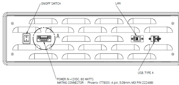
**ON/OFF SWITCH:** Controls the supply of DC power to the sm725 module.
