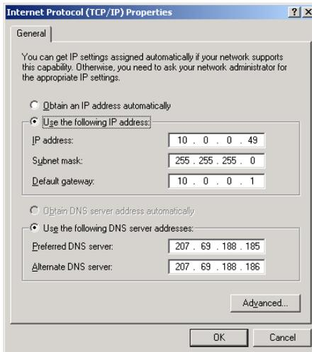
Select “Use the following IP address” and you will have access to change the IP address and subnet mask. No entries for “Default Gateway”, “Preferred DNS server” or “Alternate DNS server” are required. Click “OK” to save the settings.
