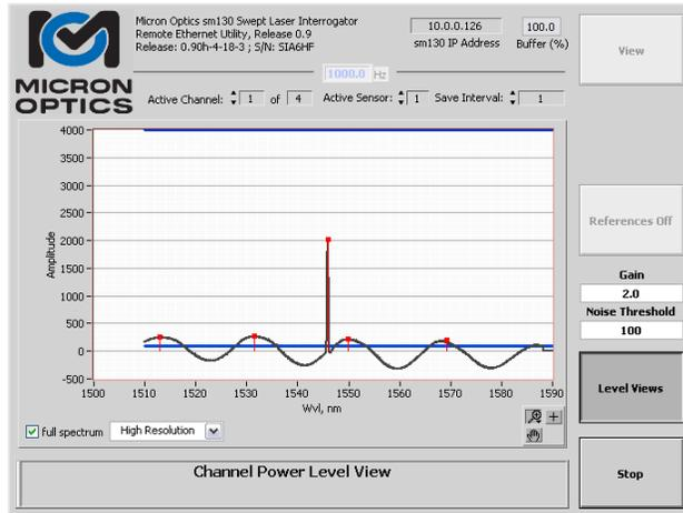
False sensor detection of PC connector back-reflection as highlighted by Spectral Diagnostic View.
