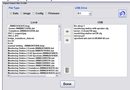
The figure above shows the Import/Export utility that manages the transfer of data from ENLIGHT to and from an external USB drive. Radio buttons on the top allow the user to choose among data, images, configuration files, and firmware file. Data transfer is facilitated by simply highlighting the desired files and clicking on the arrow control that indicates the desired direction of file transfer.
