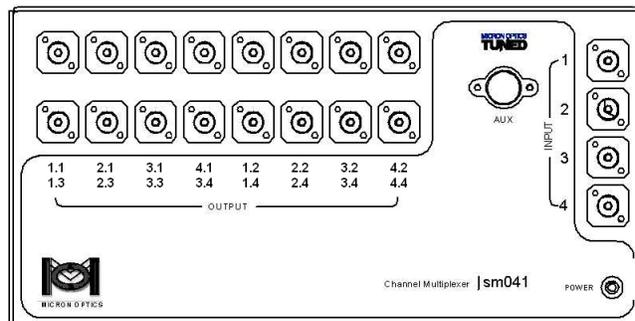
**POWER LED:** This red indicator confirms that power has been supplied to the module. A switch-type sm041 module (e.g. sm041-416) requires no separate power supply of its own, as all power and control for the multiplexer are supplied from the host interrogator module via the AUX port. A coupler-type sm041 module (e.g. sm041-016) is passive and requires only optical connectors. See INPUT and OUTPUT below.
