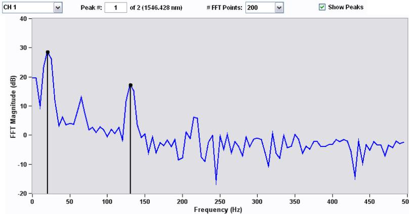
The Spectral Peak FFT View plots the frequency response of one spectral peak as measured by an x30 interrogator core. A “Channel” control and “Peak #” control select the spectral peak whose frequency response will be plotted. The “# FFT points” control selects how many sequential data points are used to calculate the FFT. The “Show Peaks” control overlays indicators of detected FFT feature in the Fourier spectrum.
