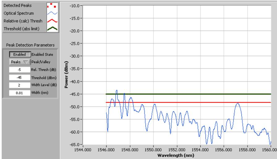
Case L: By increasing the limiting “Threshold” parameter, we prevent noise floor feature from being falsely identified as valid peak structure.
