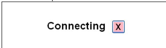
Once the configuration settings have been established, ENLIGHT will attempt to establish a constant connection with the interrogator core. During that time, a splash screen will appear, as shown in the figure above. Attempts to connect can be aborted by clicking on the red X control.
