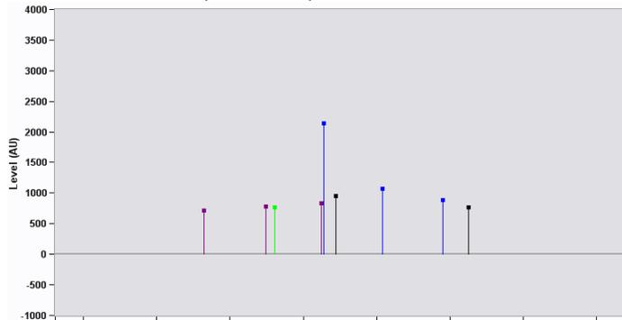
For x30 interrogator cores without the Spectral Diagnostic View feature, Amplitude View shows the count location and peak amplitude for each of the spectral peaks.
