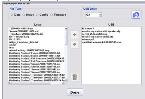
The figure above shows the Import/Export utility that manages the transfer of data from ENLIGHT to and from an external USB drive. Radio buttons on the top allow the user to choose among data, images, configuration files, and firmware file. Data transfer is facilitated by simply highlighting the desired files and clicking on the arrow control that indicates the desired direction of file transfer.
