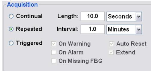
This collection of controls governs how data is collected during the time between the Start and Stop conditions.
