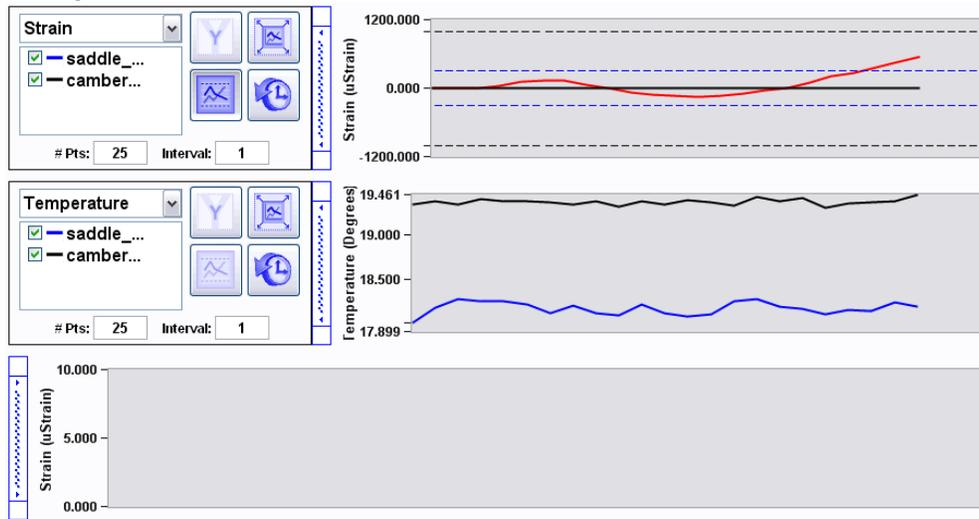
When a sensor goes into warning or alarm condition, the color of that sensor plot on the chart turns from its predefined color to either yellow or red, respectively. In the above figure, it can be seen that the “saddle\_strain” sensor has exceeded its maximum limit value and is thus in an alarm state. As such, the color of its trace has turned from blue to red.
