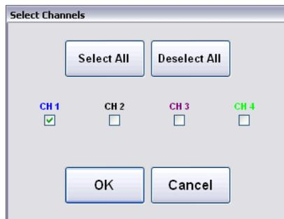
When a Create FBGs operation is initialized, a Select Channels popup window launches. A series of Boolean checkboxes offer the user control of which channels to select for automatic FBG bin creation, with the currently active channel pre-selected. "Select All" and "Deselect All" buttons offer a convenient means of mass channel selection. In the case that a multiplexer is employed in a configuration, the Select Channels window scales appropriately.
