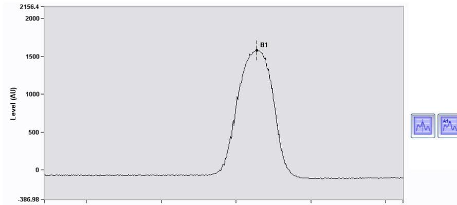
The above plot shows a spectral section (solid black line) that results in a spectral peak (dashed vertical black line) and a defined FBG (black dot with black text label).
