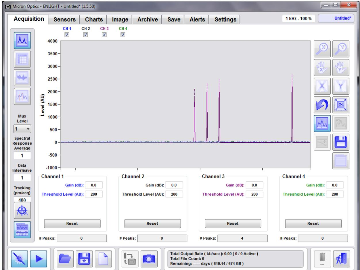
The preceding figure shows a full screen shot of MOI ENLIGHT with the Acquisition tab selected. Note that a large portion of the screenshot is filled with a tab control structure. This tab control dictates what features of the software are displayed based upon the tab selected. Note also that several controls and indicators are located outside of that tab structure. These features are visible on the GUI independent of the tab control state. The following section will detail those features.
