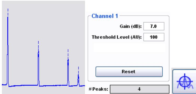
If the new peak is an intended component of the measurement system, then the “Reset Wavelength Tracking” control can be used to create a corresponding entry among the tracked peaks collection. Peak tracking has also been implemented for x25 cores.
