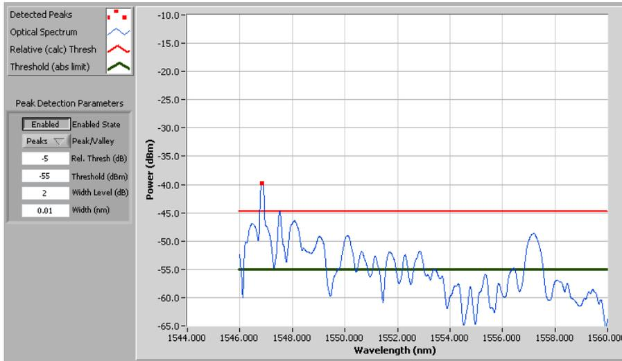
Case J: By using the relative threshold parameter, 30 dB of signal attenuation is accommodated in the PD algorithm. This is a good thing. Effective threshold is still dictated by the peak level and relative threshold, as they are above the limiting “threshold” parameter.
