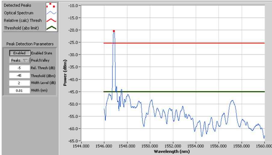
Case N: With attenuation returning towards zero, the calculated threshold continues to track 5dB below the peak amplitude. Since its value of 25dBm is greater than the limiting “threshold” values of -55dBm, the calculated relative threshold continues to function as the effective threshold, used in the PD. The updated “threshold” value of -45dBm remains to protection against false positive findings in the event of a future increases in insertion loss.
