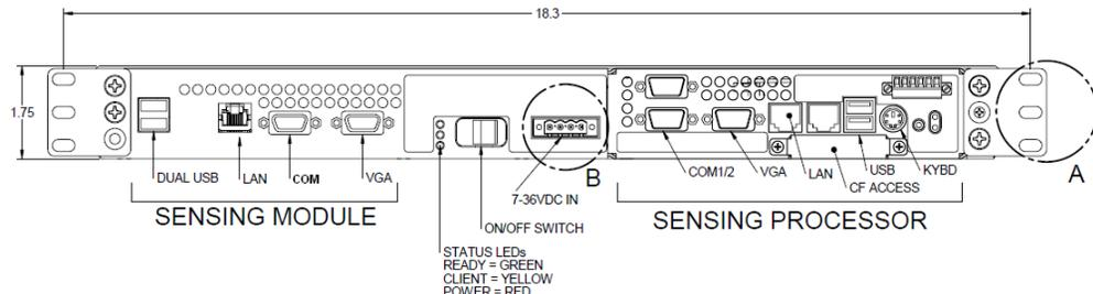
The ports for the sm225 Sensing Module are defined in the previous section. Addition of the Optional Internal Sensing Processor adds the following ports and connections.
