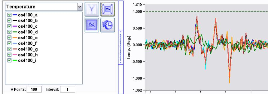
In the image above, ENLIGHT plots the Rate of Change for each of the nine os4100 relative temperature sensors and applies a positive limit of 1. An alarm will be triggered if any one of the nine sensors changes more than one degree C in a single acquisition.
