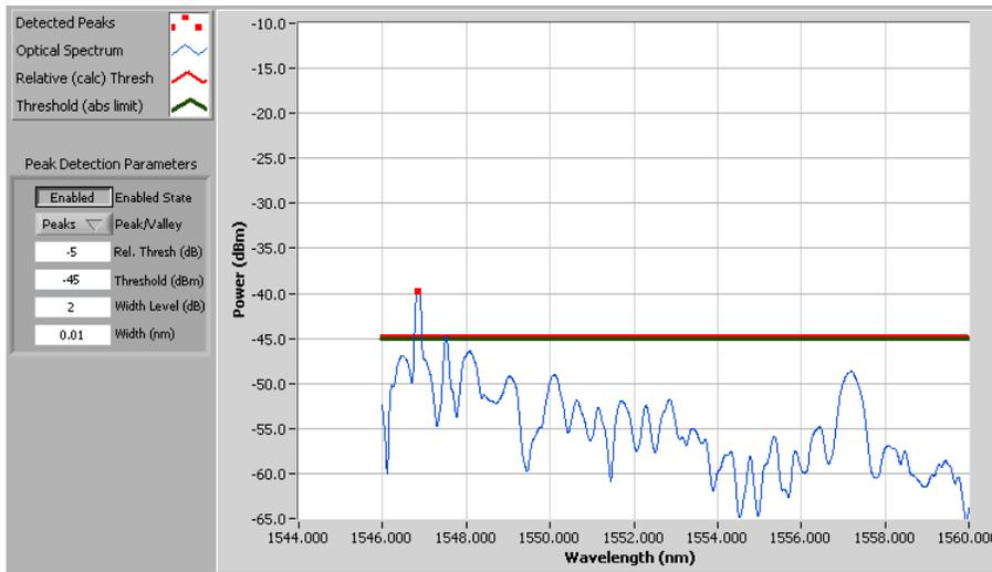
Case M: With “Threshold” set at -45, attenuation of the FBG is decreased, and the relative calculated threshold increases above the “threshold” limit...the higher of the two lines is applied as the effective threshold.
