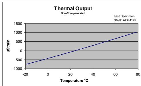
There are several methods of determining the thermal output of a gage. Once the thermal output is known, the mechanically induced strain can easily be calculated by subtracting the thermal output from the strain measured by the active gage as follows: (Note the introduction of a scaling factor that more conveniently expresses strain in units of  $\mu\text{m}/\text{m}$ )
