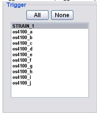
This collection of controls governs which sensors are monitored for trigger events to initiate a triggered data saving acquisition.
