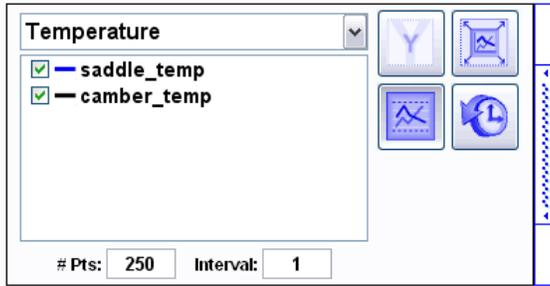
To the left side of each visible strip chart is an expanding control dock. When the dock is closed, the controls are hidden and the chart expands in the horizontal to fill the available space. When the user clicks on the blue vertical dock expansion tab, the controls again become visible and the chart constricts accordingly.
