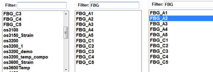
The Filter control helps users to quickly find and access target FBG or sensor elements among the complete collection of Data Archive elements. All defined FBG and sensor names stored in the ENLIGHT Data Archive are displayed in an archive elements list indicator on the Archive tab. The user can quickly locate specific subsets of FBG or sensor elements by typing a name in the Filter.
