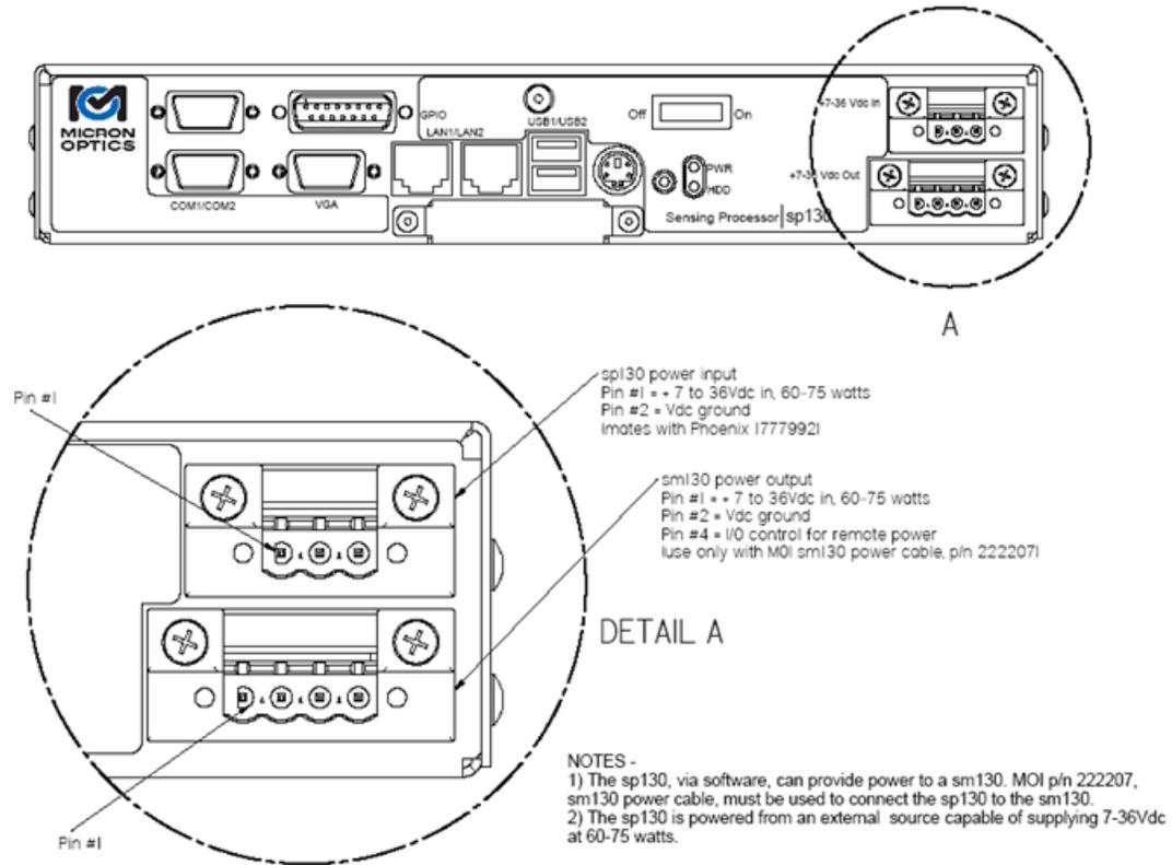
ii. General Purpose Input/Output (GPIO) Wiring Diagram
