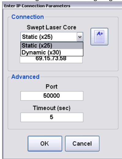
In a desktop or stand-alone installation, the user will be asked to choose the type of target module and configure ENLIGHT with the correct TCP/IP settings. Once the parameters are selected, ENLIGHT allows the user to check the settings with the “Test” button, pictured above as the icon with the “A+”. ENLIGHT will then attempt to make a connection to the interrogator as configured by the user and will inform the user whether or not the connection was successful via a pop-up message.
