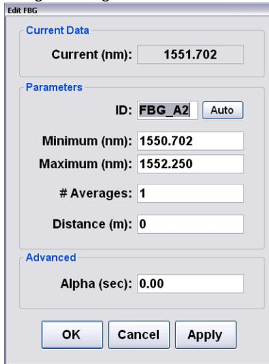
The preceding data entry form is used to set/modify the attributes for the selected FBG. This form is launched by both the “Add FBG” and “Edit FBG” buttons, as well as a double click event on one of the FBG entries on the table, in the case of desktop deployments.
