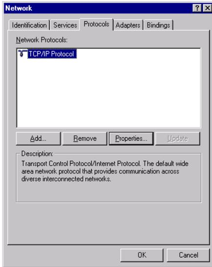
Click on the tab labeled “Protocols” and highlight the “TCP/IP Protocol”. Click on “Properties” and the following window will open.
