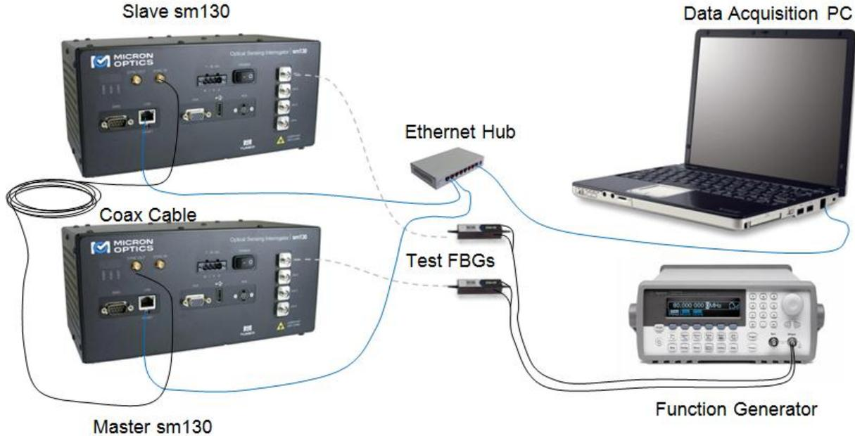
Hardware configuration for synchronized test measurement.
