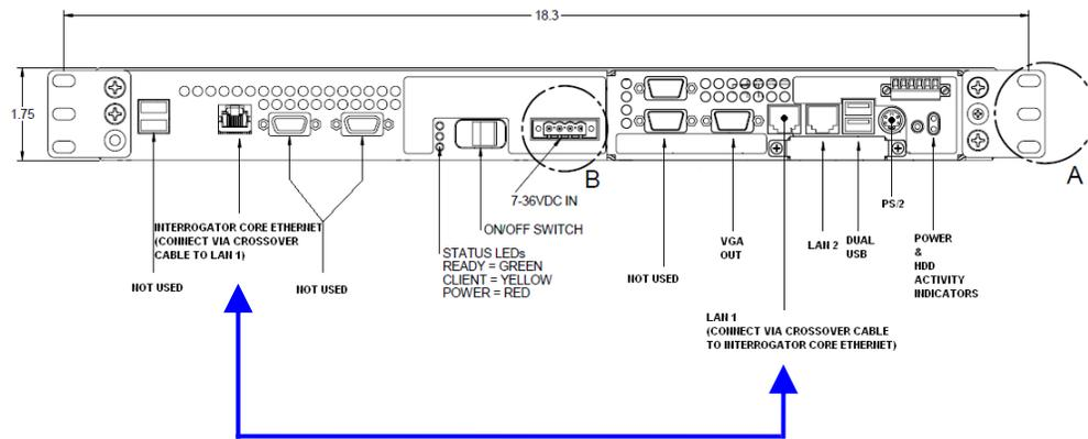
**CRITICAL NOTE: Ethernet crossover loopback connector REQUIRED for operation.**
