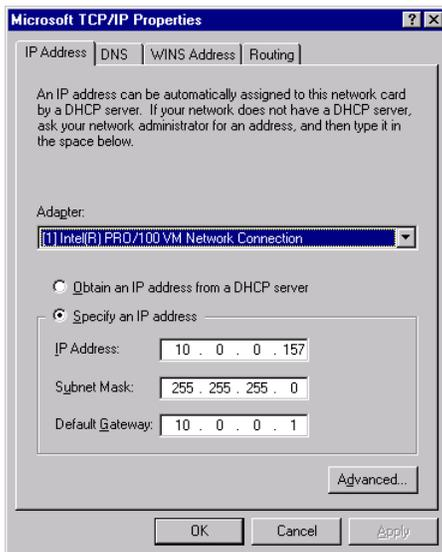
Choose “Specify an IP address” and you will have access to change the subnet mask and IP address. No entry for “Default Gateway” is required. Click “OK” to save settings.
