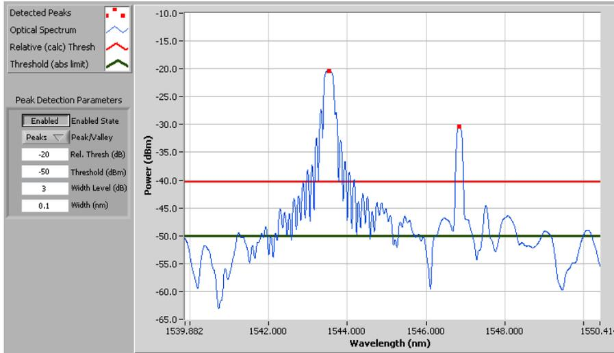
Case G(1). First method for isolating signals from side modes. Keep evaluation of peak width at 3 dB bandwidth and change the required bandwidth, such that narrower side modes do not meet the criteria, but fundamental FBG modes do.
