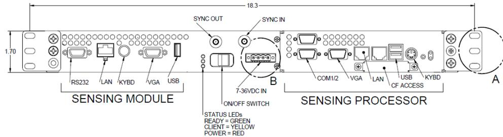
The ports for the sm230 Sensing Module are defined in the previous section. Addition of the Optional Internal Sensing Processor adds the following ports and connections.
