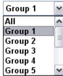
Allows the user to display a configurable subset of the full sensor collection by selecting one of the preconfigured groups. Sensors can be assigned to a group using the Edit Sensor window. Ten independent groups are provided for organizing and filtering sensor collections.
