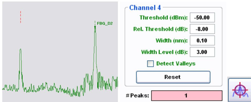
Following the example further, it is seen that the first spectral peak on channel 4 (which corresponds to FBG "FBG\_D1") has fallen below the Rel. Threshold Level of -8 dB. With this information, the user can either seek to correct the root cause of the attenuation or change the peak detection parameters in order to re-enable detection of the missing spectral peak.
