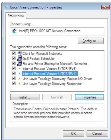
Right click on the Internet Protocol Version4 (TCP/IPv4) entry and select “Properties”. The following window will open, allowing for change of the default IP address and Netmask of the PC.
