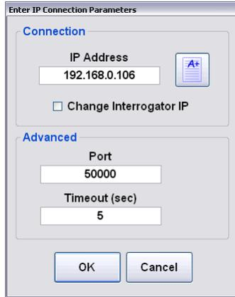
When already connected to an Interrogator core, the IP address of that core can be changed by updating the IP Address field and checking the “Update Interrogator” checkbox. After clicking “OK”, the x25 or x30 core will reboot in order to facilitate the change of IP address, and a socket connection will be re-established with the interrogator core on the new, updated IP address.
