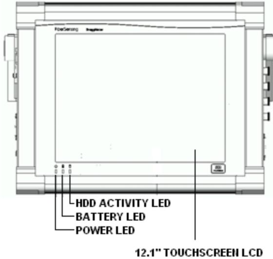
**12.1" TOUCH SCREEN LCD:** The 12.1" touch screen LCD is the primary data input and GUI display device for the si325 interrogator. Text input is facilitated by an on-board virtual keyboard.
