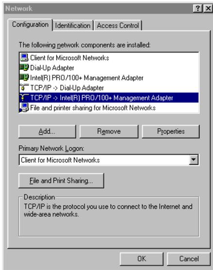
Highlight the appropriate TCP/IP adapter and click “Properties”. The following window will then open.
