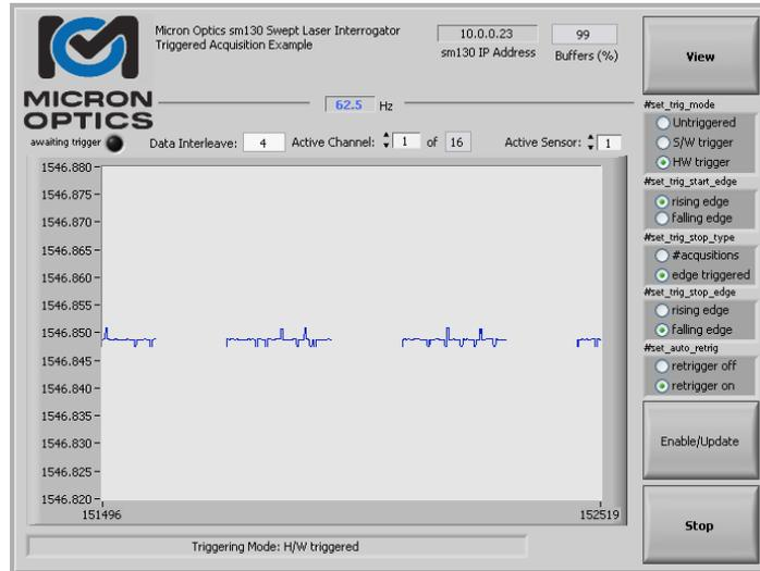
Hardware triggering configured for rising edge start, falling edge stop, with automatic retrigger off.
