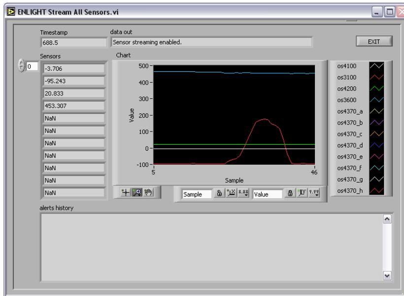
The third functional tab launches a sub-routine that exercises some of the streaming data commands to facilitate a continuous, buffered stream of calibrated sensor data from the ENLIGHT RCI to the LabVIEW client.
