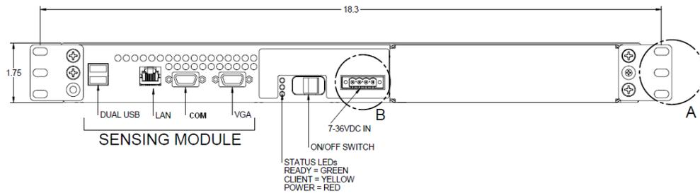
**POWER LED:** This red indicator confirms that power has been supplied to the module.
