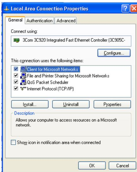
Highlight the “TCP/IP” entry and click “Properties”. You will then have access to change the IP address and subnet mask. Click “OK” to save settings.
