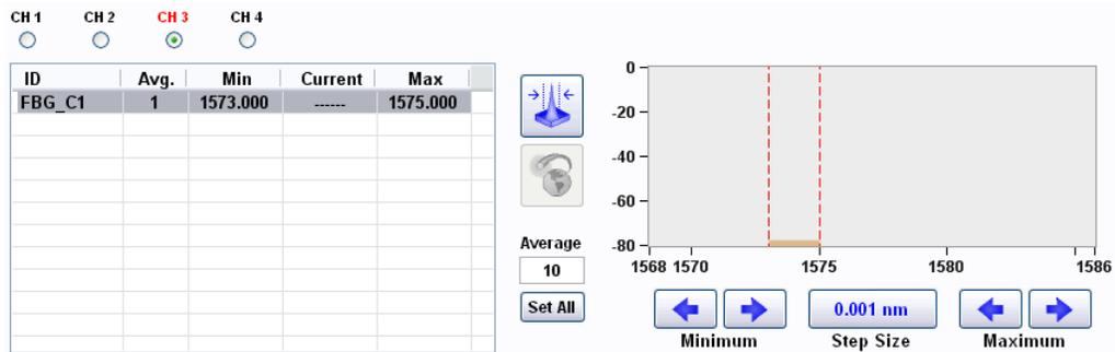
The absence of the grating is indicated by the red bin limits and channels 3 label, but sensors can still be created from the FBG\_C1 reference.
