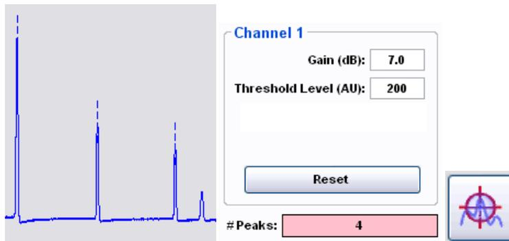
The preceding graphic shows a condition where a spurious peak has been introduced to the sensor system, and has been detected by the x30 interrogator. In this example, the three tracked and detected peaks are indicated by the blue vertical lines. The red-highlighted “# Peaks” indicator shows that a total of four peaks have been detected, though only three have been tracked. This fourth peak will not be included in any subsequent FBG or sensor definitions unless included among the tracked peaks.
