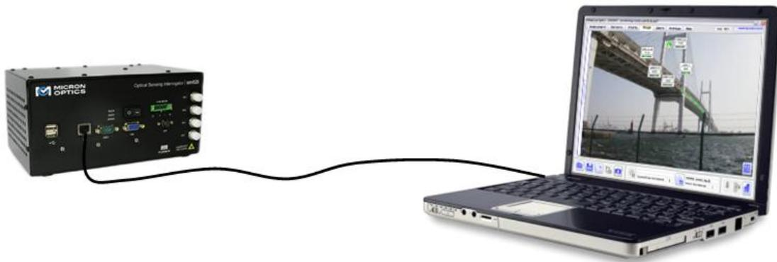
**sm125 Optical Sensing Interrogator Module**
