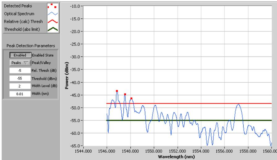
Case K: With several more dB of attenuation and still using relative threshold, the PD algorithm begins to get false positives, by identifying noise structure as valid peaks. This is why the absolute “threshold” parameter is included. It should be used to prevent massive attenuations from resulting in false positive numbers.
