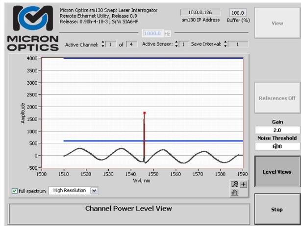
Use of the Noise Threshold Level control to eliminate false sensor detection
