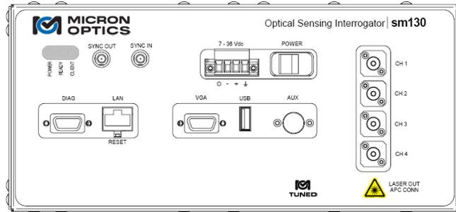
NOTE: The only required peripheral for normal operation is an RJ-45 Ethernet Cable.
