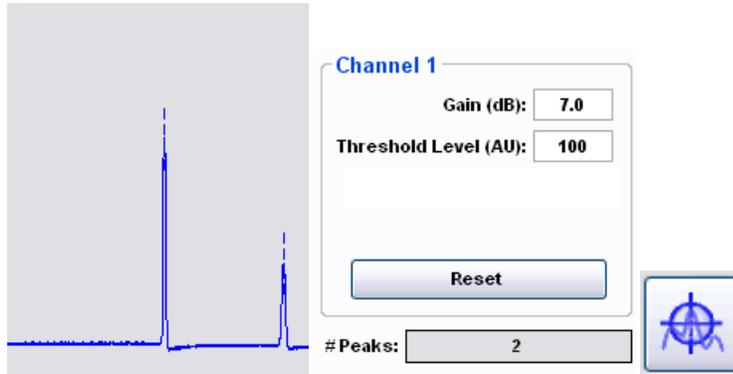
**Case II.** An additional peak is introduced to the system, yielding a greater number of detected peaks than tracked peaks.
