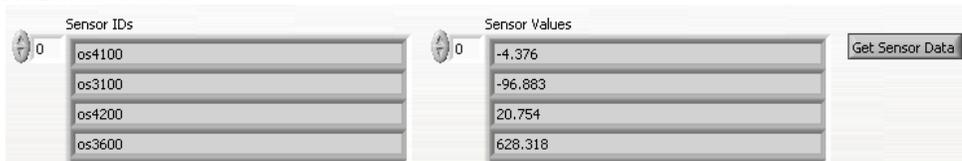
The next functional tab demonstrates how to extract a single, un-buffered collection of sensor IDs and sensor values. This tab exercises the #GET\_SENSOR\_ID and #GET\_SENSOR\_VALUES commands to return the latest data sets when the Get Sensor Data button is pressed.
