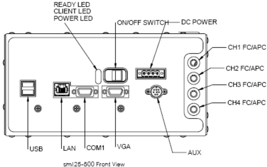
**ON/OFF SWITCH:** Controls the supply of DC power to the sm125 module.
