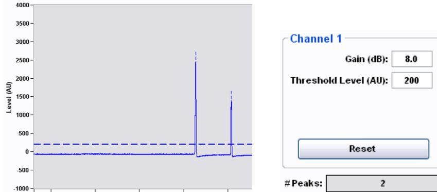
Note the transient dashed line that appears for 1 second to indicate that the Noise Threshold value is changed. This indicator also appears briefly when the Gain control is changed. Dashed lines also indicate threshold settings for x25 interrogator cores.
