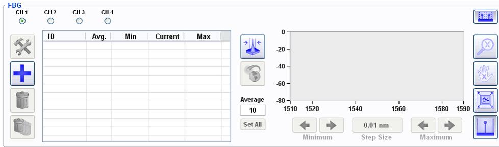
The top half of the Sensors tab is equipped with the tools to create and manage FBG elements.
