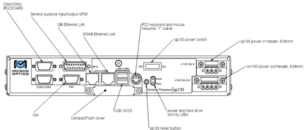
**VGA:** Used for connection to an external VGA monitor.
