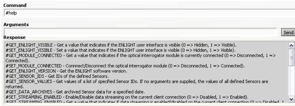
The first functional tab demonstrates a basic command utility for the ENLIGHT RCI. The “Command” and “Parameter” controls are used to send a parameterized command to the RCI and display the response below.
