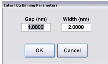
The user enters data to define the desired maximum “Width (nm)” of the spectral bins and the minimum acceptable “Gap (nm)” between bins. MOI ENLIGHT then automatically defines wavelength bins for each FBG according to the requirements.
