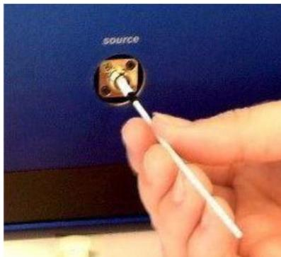
Figure 7-5 - Cleaning Optical Bulkhead Connections
