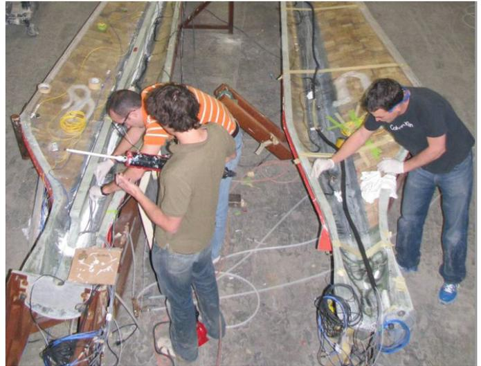
Sensing system installed inside SBlade
