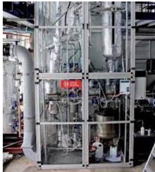
Heat Exchanger for Condensing Hexanol
