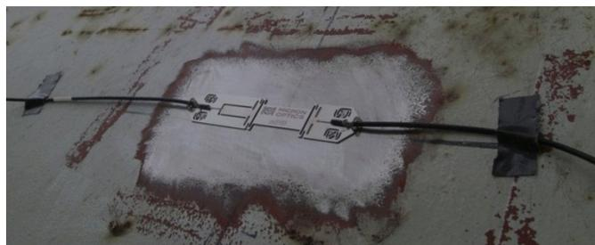
Luna's os3155 rugged fiber optic strain gages are installed along exterior steel plate girders to measure strains for loads that can run as high as 410,000 lbs.
