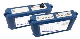
The OBR 6225-2 (top) incudes a sealed, dual FC/APC connector, while the OBR 6225-1 includes a single standard FC/APC optical connetor.
