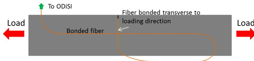
Figure 4: Fiber bonded strategically on test article
