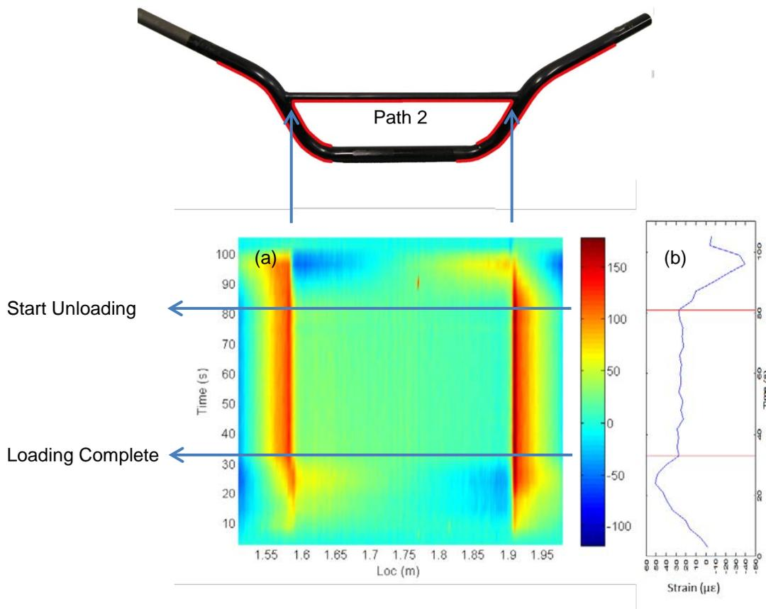
Figure 7. (a) The strain of path 2 shown over time. (b) Strain at 1.63 m along the sensor over time.
