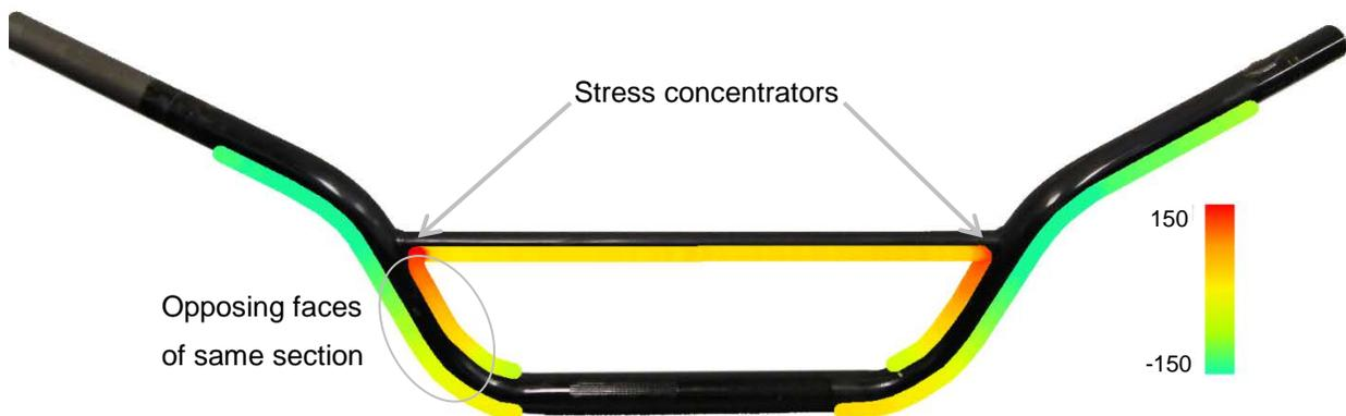
Figure 5. Strain along the fiber superimposed on handle bar image. Color bar = strain range in microstrain.
