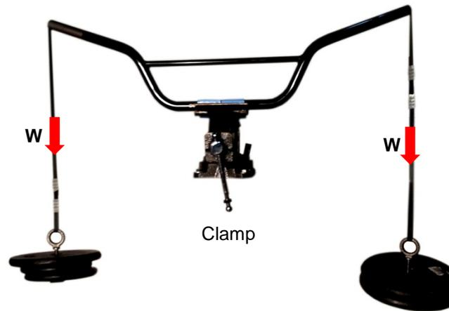
Figure 3. Experimental setup. The handle bar is held steady with a clamp, and weights are suspended from each handle bar.
