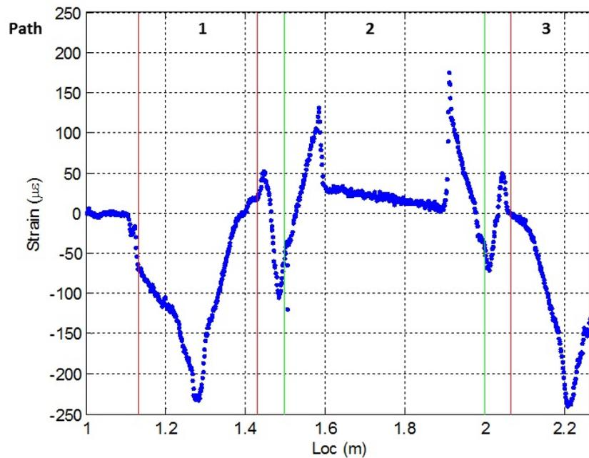
Figure 4. The strain along the sensor at maximum load. Each path of the handle bar is outlined on the graph by vertical lines.
