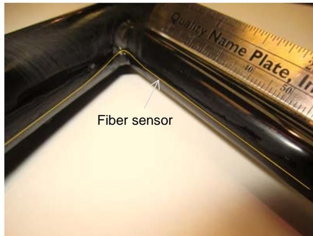
Figure 2. Close-up of acute angle weld instrumented with fiber optic sensor.
