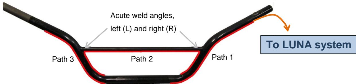
Figure 1. Red regions represent the bonded fiber paths of interest along the handle bars. The path numbers correspond to sensor paths as also labeled in Figure 4.
