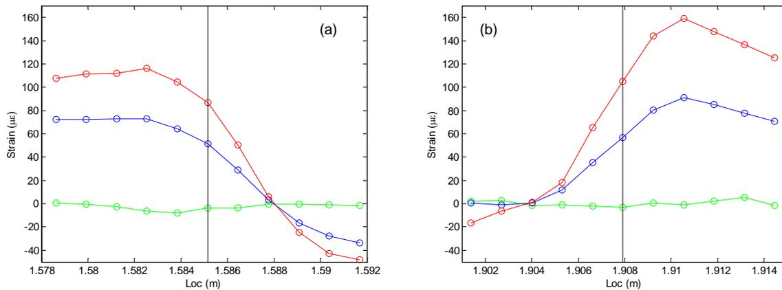
Figure 6. Strain across the weld shown at 1.25 mm spatial resolution for acute angle welds on the (a) Left and (b) Right welds, at three instances during the transition from zero loading to fully loaded. Green: zero load, blue: intermediate load, red: maximum load, black: weld location.
