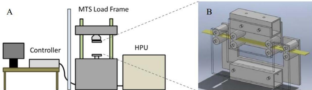
Figure 2: A. MTS load frame, controller, and HPU. B. Custom four-point-bend test fixture.
