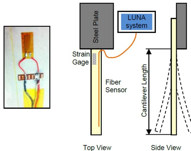
*Figure 1: Schematic of fatigue test setup for experiment one.*
