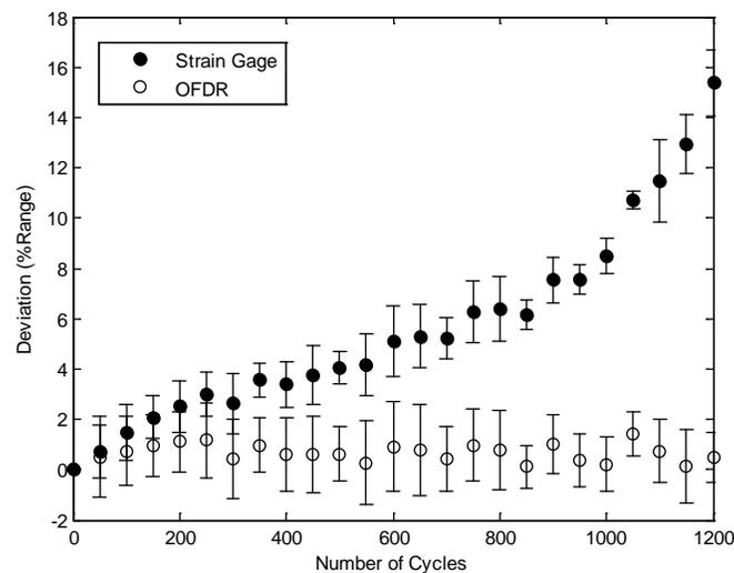
Figure 4: Percentage deviation of strain measurements with number of cycles for a single coupon.
