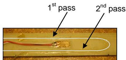
Figure 3: Fiberglass coupon instrumented with a foil strain gage and two passes of fiber optic sensor.
