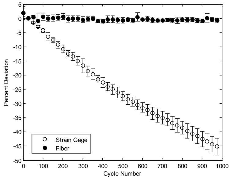
Figure 5: Percentage deviation of minimum strain for each cycle, from initial minimum strain.
