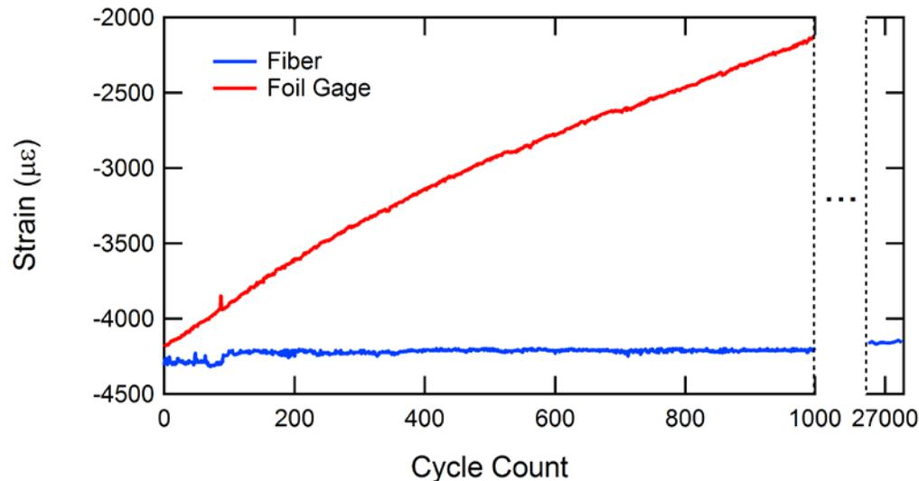
Figure 6: Strain as a function of number of cycles. The foil gage suffers from severe drift where the fiber sensor continues to measure accurately up to over 27,000 cycles.
