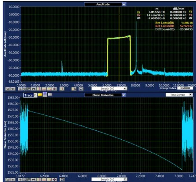
Figure 1: Phase Derivative (Wavelength) of Grating Versus Distance
