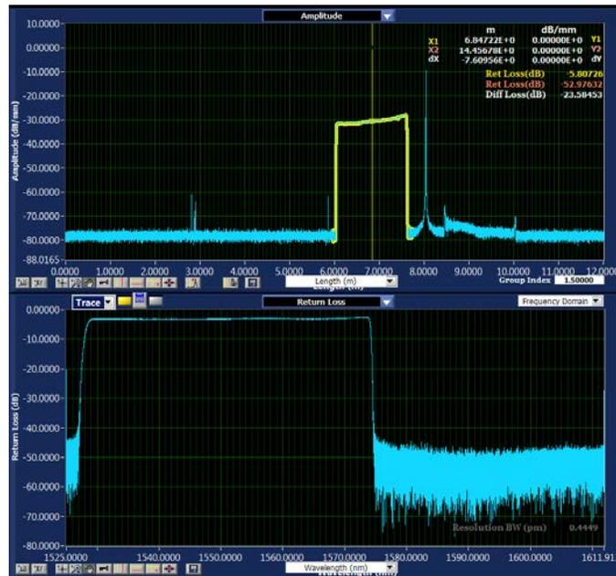
Figure 2: Return Loss of Grating as a Function of Wavelength
