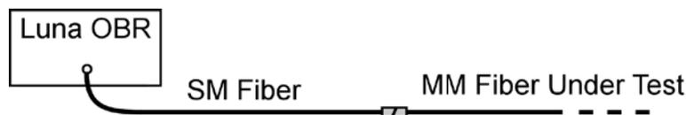
*Figure 3. Direct launch from single mode to multi-mode fiber.*
