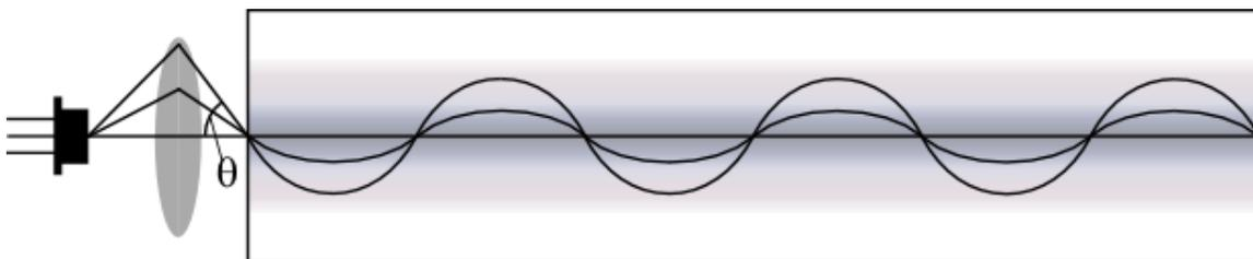
*Figure 2. Light from a packaged semiconductor light source, such as an LED, is collected by a lens and injected into a graded-index MMF. Three rays are shown: one ray along the fiber axis which depicts the lowest order mode and two rays with higher angles of incidence  $\theta$  which couple into higher order modes that travel closer to the core-cladding boundary.*
