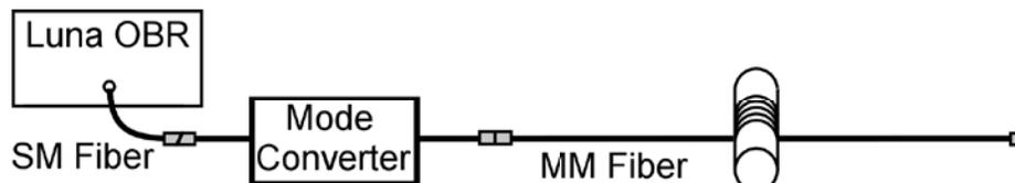
Figure 16. OBR mode scrambler launch measurement of IL due to a mandrel wrap.
