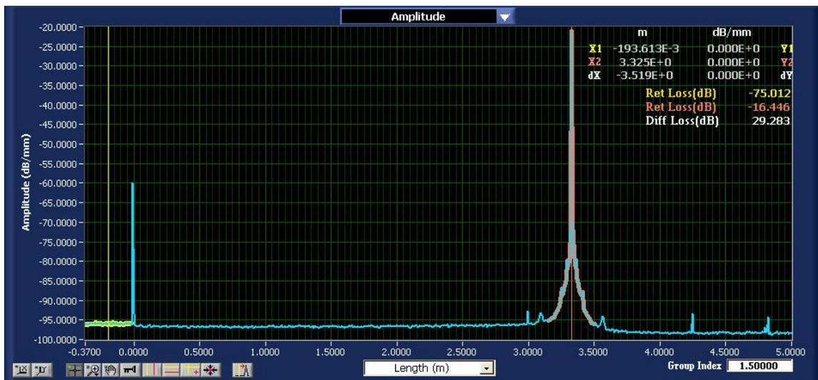
Figure 21. The OBR upper graph trace for a multi-mode jumper with a FC/PC end connector
