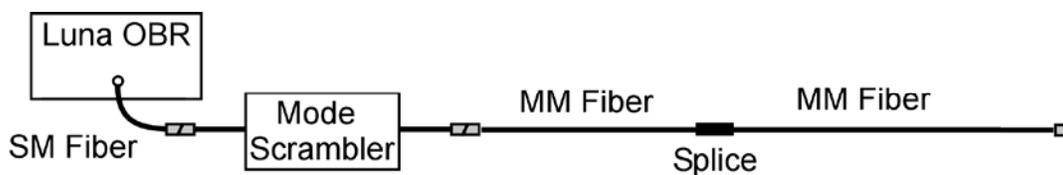
Figure 7. Network diagram of the same multi-mode jumper as in Figure 5 is connected to a mode converter which is in turn connected to the front panel of the OBR
