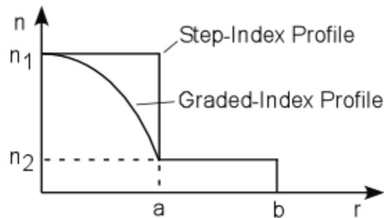
*Figure 1. Index of refraction,  $n$ , profile as a function of fiber radius,  $r$ , showing the difference between step-index and graded-index MMF. Modes are bound within the core radius  $r = a$  by the index of refraction difference between core and cladding of  $n_1 - n_2$ .*
