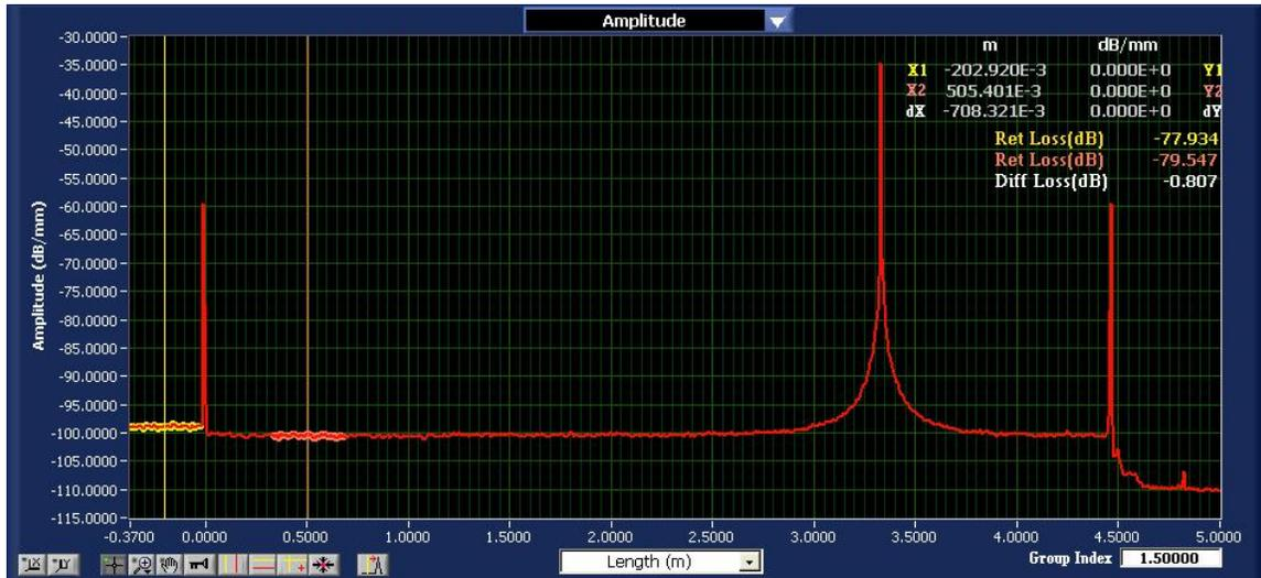
Figure 22. The OBR upper graph trace for jumper in Figure 21 with a second jumper added to reduce the reflection from the FC/PC connector so that the highest detector gain setting could be used for the IL measurement.
