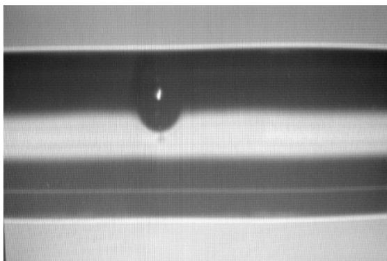
Figure 10. A splice in multi-mode fiber with a bubble near core edge.
