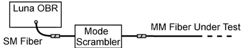
Figure 4. Mode scrambler launch from single to multi-mode fiber.
