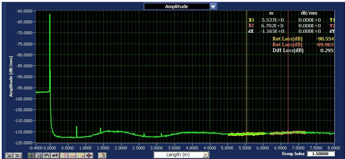
Figure 9. The OBR upper graph trace showing the instrument background noise level. The background return loss of the noise level is measured for the same cursor locations and integration width as used in Figure 8.
