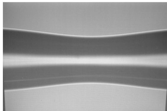
Figure 11. A splice in multi-mode fiber resulting in narrow waist.
