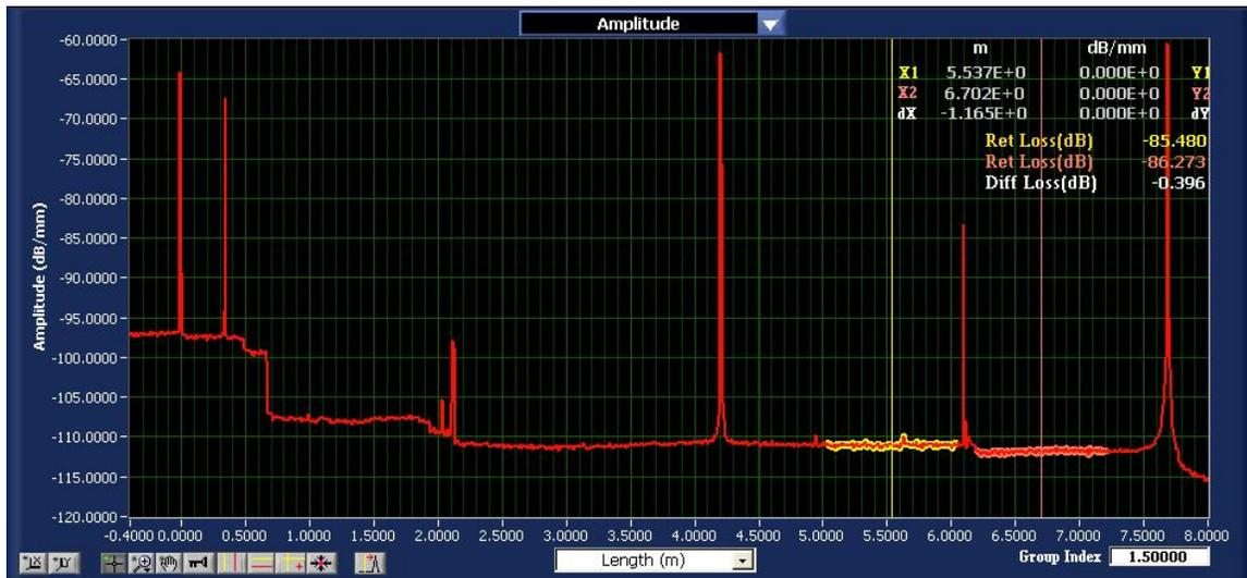
Figure 8. The OBR upper graph trace for the network shown in Figure 7 which contains the splice shown in Figure 5. An insertion loss measurement is performed by placing the vertical cursors before and after the splice and subtracting of the background noise level.
