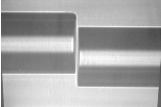
Figure 12. Offset Splice C just prior to fusion.
