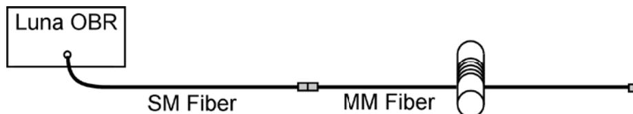
Figure 15. OBR direct launch measurement of IL due to a mandrel wrap.
