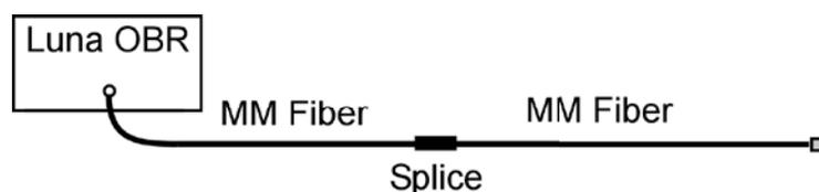
Figure 5. Network diagram of multi-mode jumper connected to the front panel of the OBR with a splice mid-way along its length.
