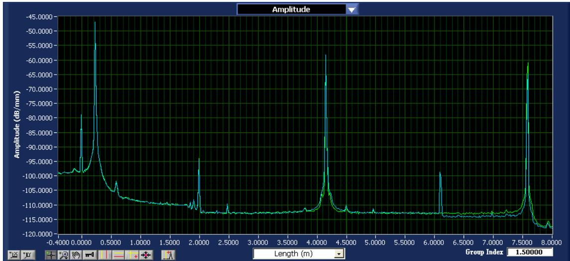
Figure 17. OBR upper traces of the network shown in Figure 16, without (blue) and with (green) a mandrel wrap consisting of one loop around a 7.5 mm mandrel.
