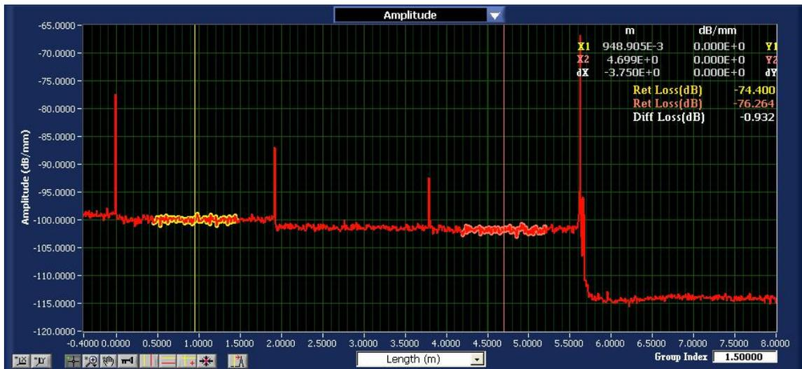
Figure 20. The OBR upper graph trace for the network depicted in Figure 19.
