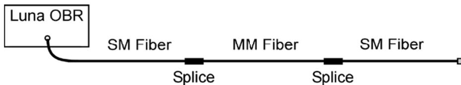
Figure 19. Jumper required for measuring relative scatter level of multi-mode fiber.
