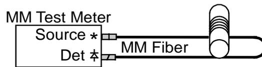
Figure 14. Multi-mode meter measurement of IL due to a mandrel wrap.
