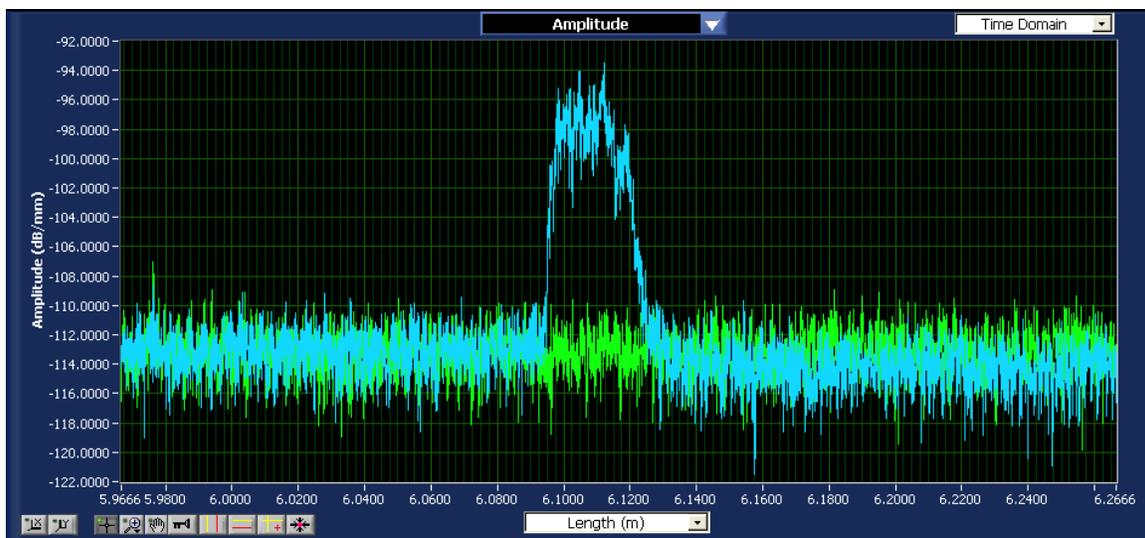
Figure 18. OBR lower trace of the network shown in Figure 16 detailing the scatter signature of the mandrel wrap in Figure 17.
