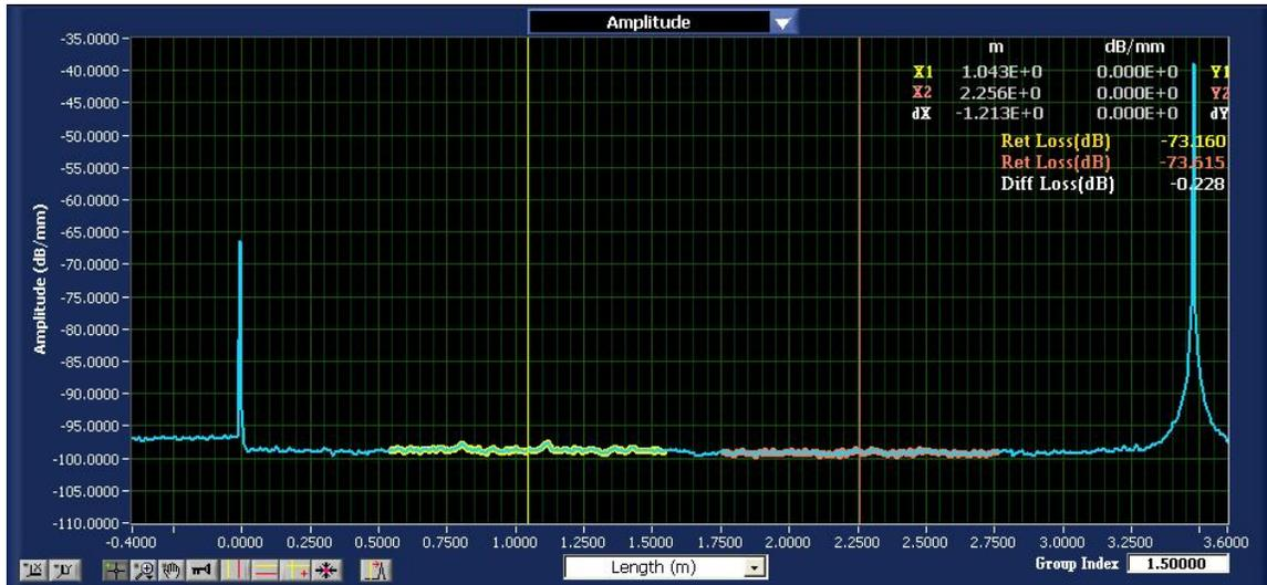
Figure 6. The OBR upper graph trace for the network shown in Figure 5. An insertion loss measurement is performed by placing the vertical cursors before and after the splice.
