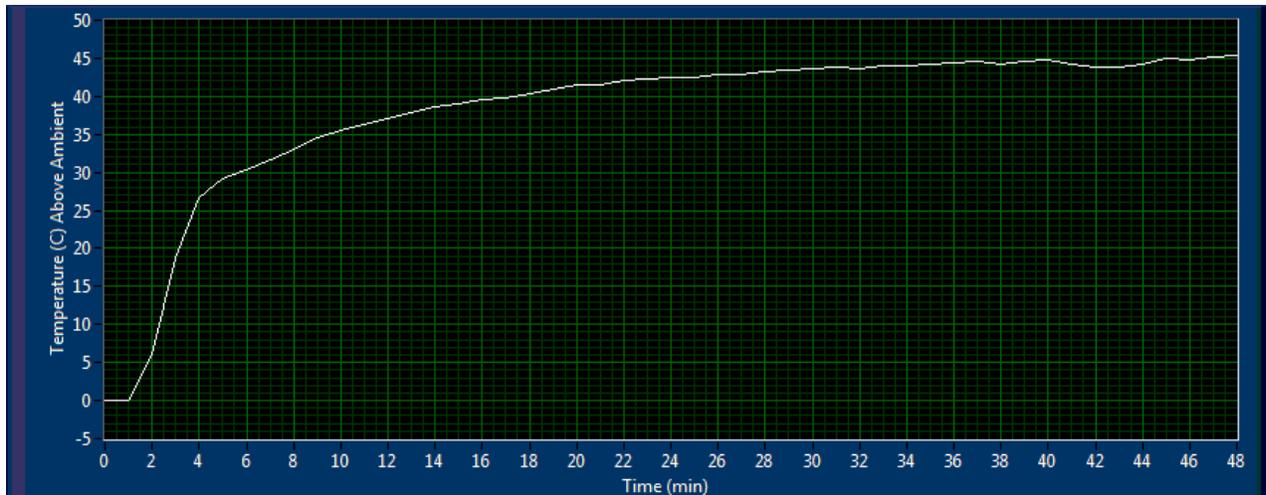
*Figure 4. Time-lapse temperature of plot of laser ADC. The temperature continues to rise even after system failure occurs after 40 minutes.*
