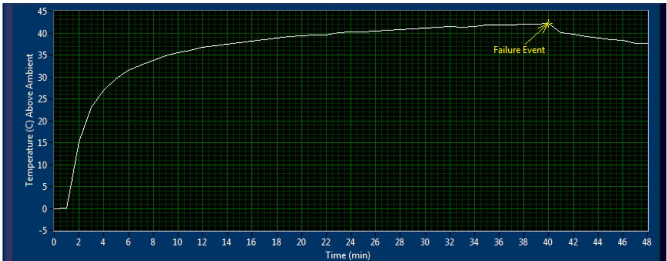
Figure 3. Time-lapse temperature plot of detector ADC 5. Again, system failure can be seen here after 40 minutes.
