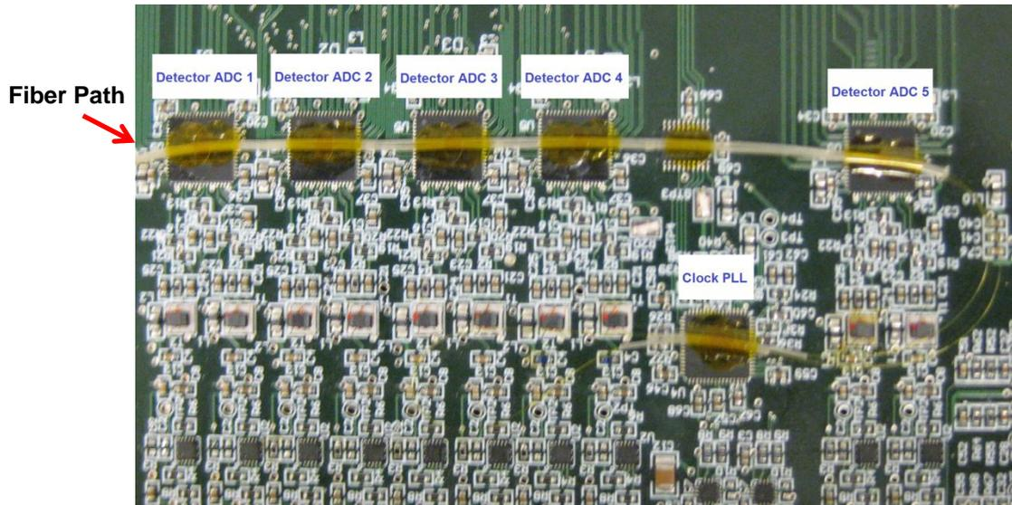
Figure 2. Sensing fiber positioned on the detector board. The fiber is routed through Teflon tubing attached to 5 ADCs, a level translator, and a clock PLL. Note that the fiber passes twice across each chip.
