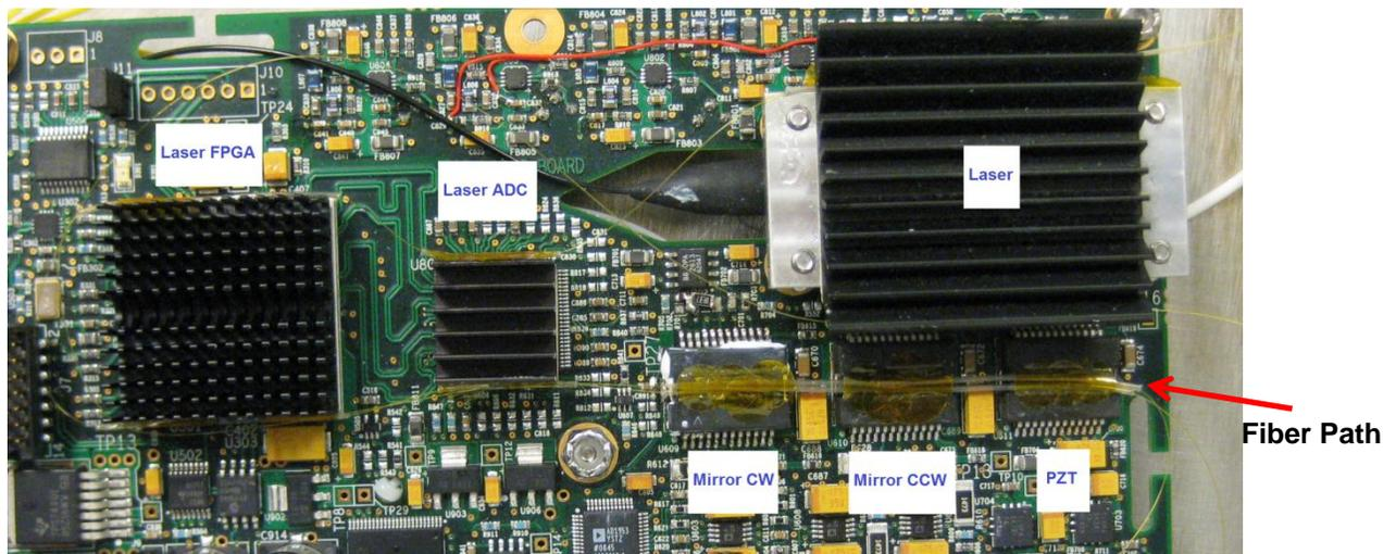
Figure 1. Sensing fiber positioned on laser board. The fiber is routed through Teflon tubing attached to the laser, the laser ADC, the laser FPGA, and three op-amps. Note that the fiber passes twice across each chip.
