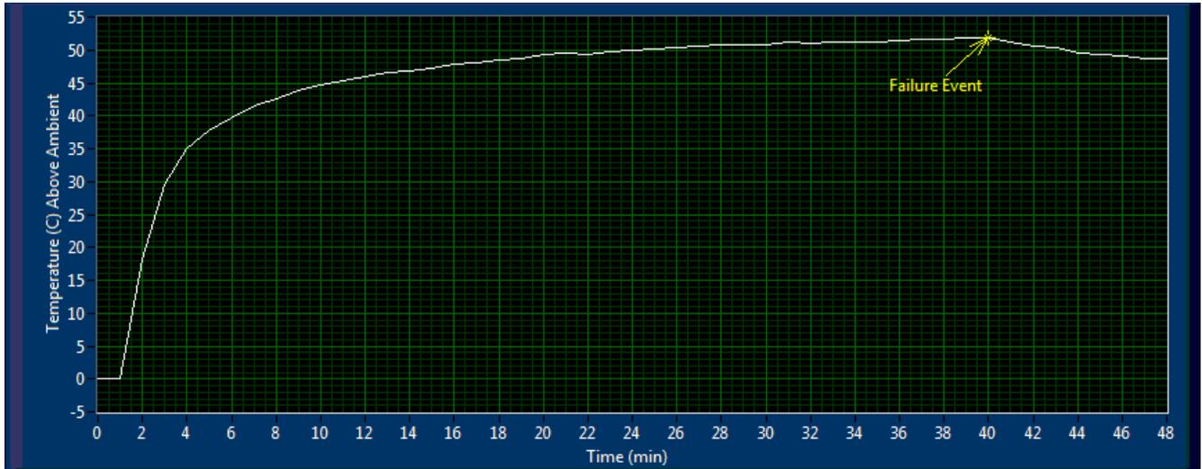
Figure 2. Time-lapse temperature plot of the Clock PLL. System failure occurs after 40 minutes.
