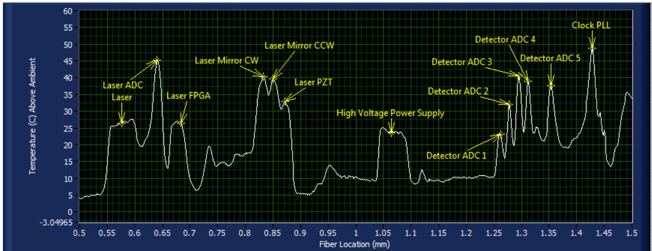
Figure 1. Temperature plot (degrees C above ambient) of the first 1.5 m of sensing fiber. The peaks correspond to the components of interest and are labeled accordingly.
