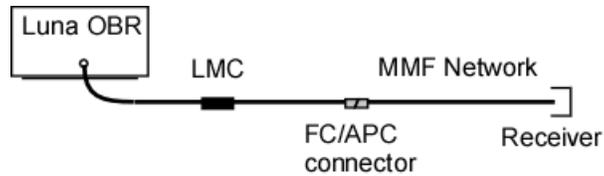
Figure 4. Measurement setup used to locate fault in MMF network branch
