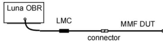
*Figure 2: Example mode conditioned launch measurement network. The output of the Luna Mode Conditioner (LMC) is FC/APC so the MMF DUT should be connectorized with a FC/APC connector (as shown) or spliced directly.*
