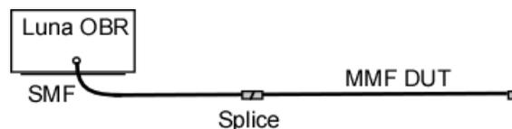
*Figure 1: Direct launch measurement network. The bulkhead connector on Luna's OBR is FC/APC, therefore in a direct launch setup the multi-mode device should be connectorized with a FC/APC connector or spliced directly (as shown).*
