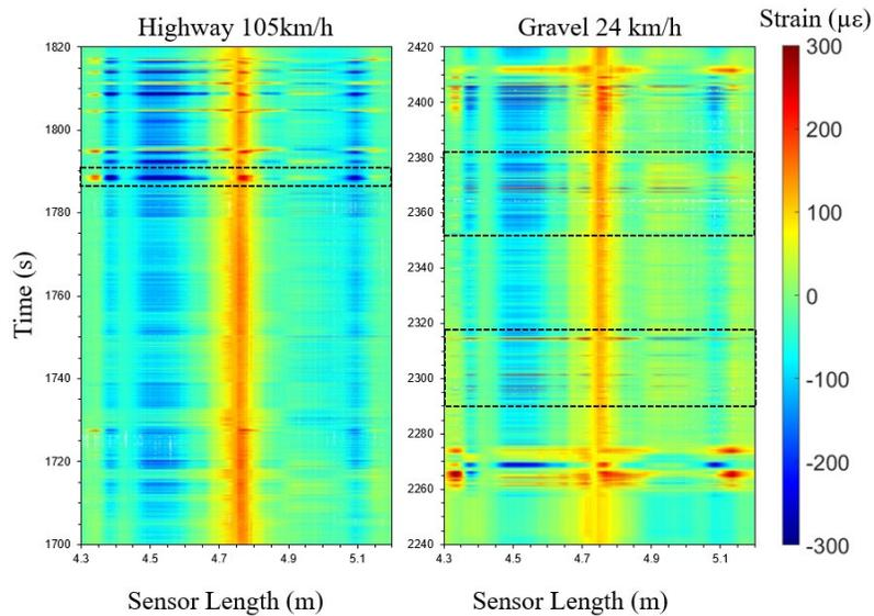
Figure 5. Right control arm strain comparison for highway and gravel road results. The highway data was very stable and clearly shows braking events, an example of which is enclosed by dashed lines. Driving on the gravel road resulted in greater strain shifts from impacts with bumps and holes as well as noisier data than the highway. These bumpy sections are enclosed in the dashed lines.
