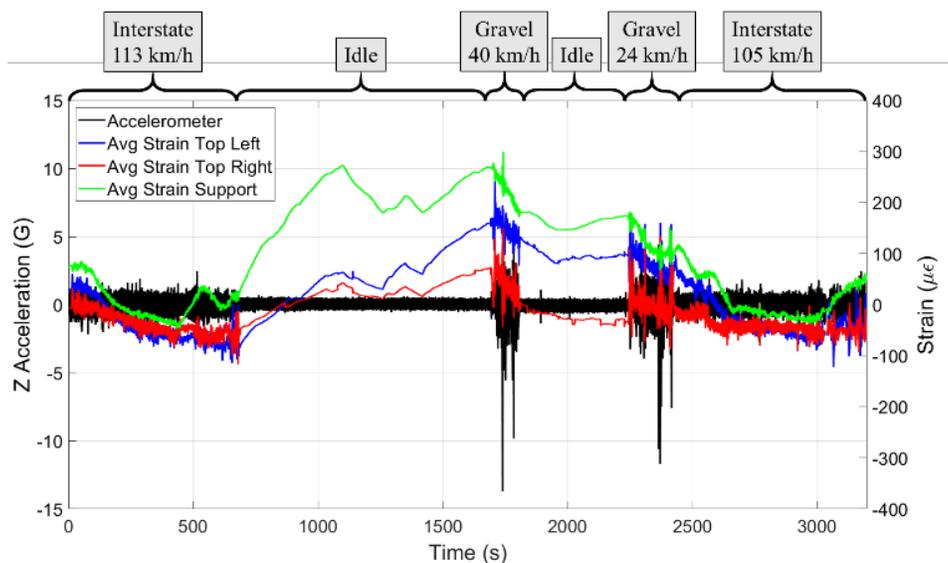
Figure 4. Accelerometer and strain measurement correlation. Z axis accelerometer data clearly shows the duration of interstate and service road conditions. The average strain for the top segments of both control arms and the support beam show corresponding times of activity. The rise in strain in between dynamic events was due to heating under the vehicle during engine idle.
