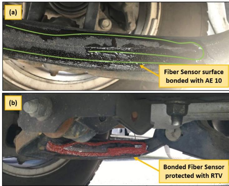
Figure 2. Bonding method for sensor instrumentation. The fiber makes two passes on its control arm, at the top and bottom of the inner curved surface.
