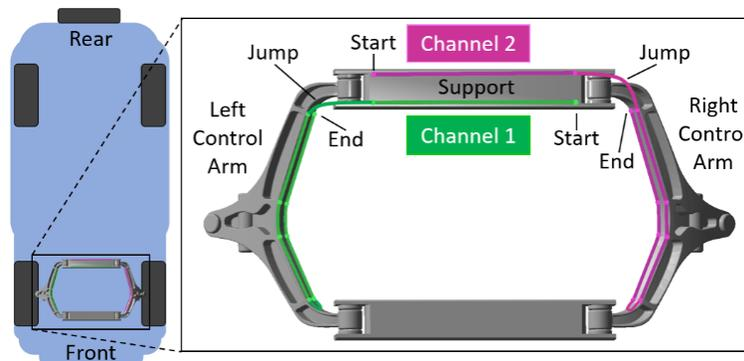
Figure 1. Instrumentation location underneath the vehicle. Two sensors were used to monitor the support beam and control arms on both sides of the vehicle. Channel 1 and 2 were instrumented in opposite directions on the support beam but identically on the control arms.
