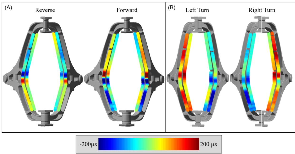
Figure 3. CAD of left and right control arms braking (A) and turning (B) with strain map overlay.
