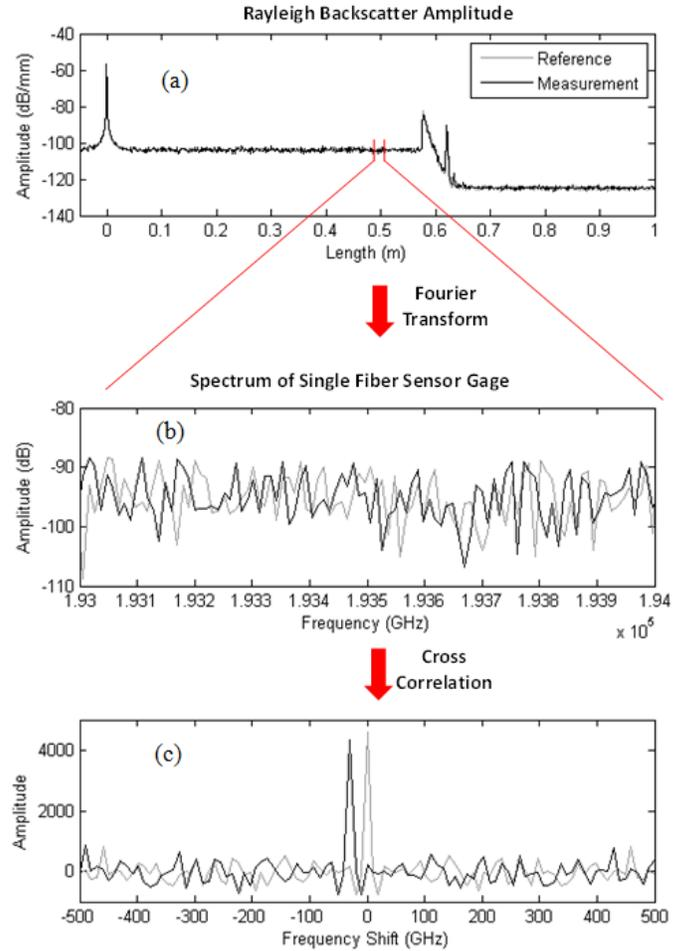
**FIGURE 2. FREQUENCY SHIFT CALCULATION FROM RAYLEIGH SCATTER MEASUREMENT. (A) RAYLEIGH BACKSCATTER ALONG OPTICAL PATH. (B) SPECTRUM OF SINGLE SENSOR GAGE. (C) CROSS-CORRELATION OF REFERENCE AND MEASUREMENT SPECTRA. [12]**
