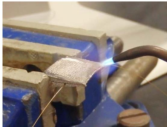
**FIGURE 15: SAMPLE FIXTURED IN A SMALL VICE AND BEING HEATED WITH AN OXY-PROPANE TORCH.**
