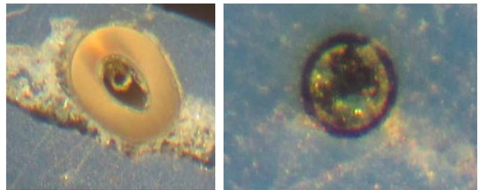
**FIGURE 4: SECTION VIEW OF THE REGION WITH PTFE TUBING CONTAINING FIBER (LEFT). SECTION VIEW OF FIBER DIRECTLY EMBEDDED INTO THE MATERIAL.**
