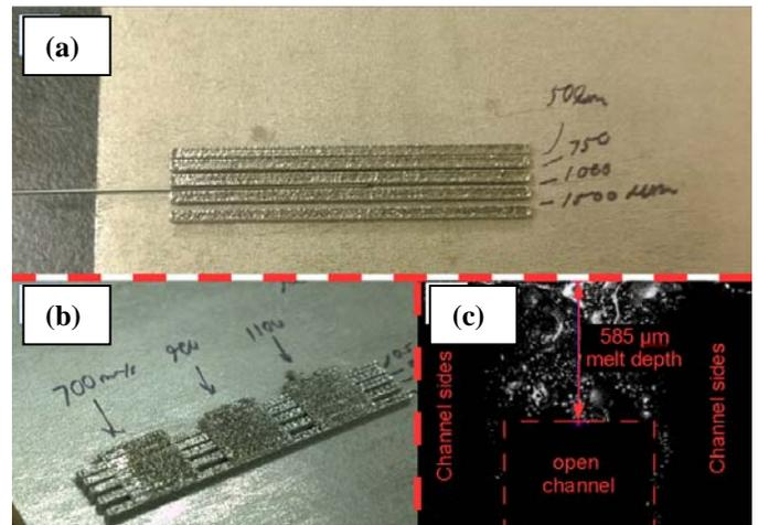
**FIGURE 9: ITERATIONS PERFORMED TO DETERMINE THE CHANNEL PARAMETERS.**
