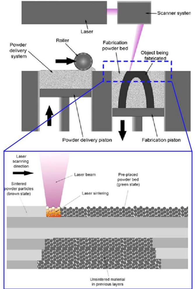
**FIGURE 7: SCHEMATIC OF THE SLM PROCESS**
