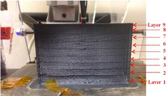
**FIGURE 6: COMPLETED BLOCK WITH 9 LAYERS CONTAINING OPTICAL SENSING FIBER.**
