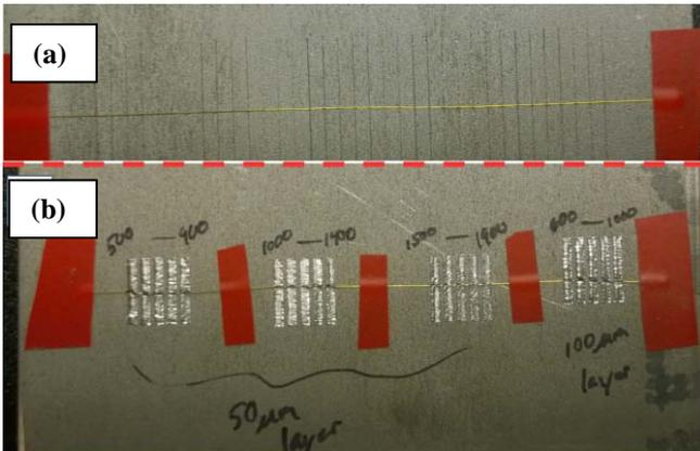
**FIGURE 8: TESTS CONDUCTED TO DETERMINE THE APPROPRIATE POWER LEVELS FOR THE SLM SYSTEM.**
