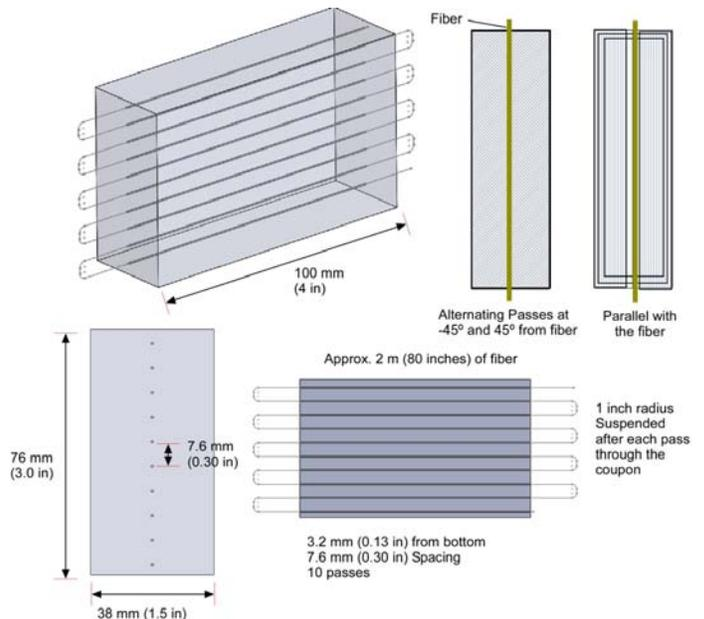
**FIGURE 5: DESIGN OF THE LARGER ABS BLOCK USED FOR RESIDUAL STRAIN TESTING.**
