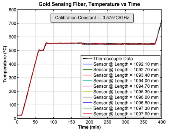
**FIGURE 14: DATA FROM THERMAL STABILITY TESTING AT 550 °C OVER A 5 HOUR TIMEFRAME.**
