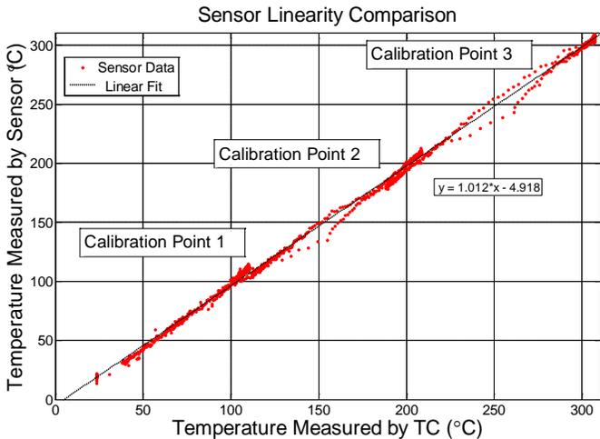
**FIGURE 13: DATA FROM THE 300°C TEMPERATURE CYCLE USED FOR ACCURACY DETERMINATION.**
