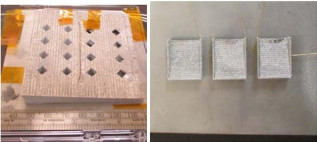
**FIGURE 10: CONCEPTUAL IMAGES SHOWING THE APPROXIMATE LOCATIONS OF THE FIBER WITHIN THE SAMPLES (TOP). COMPLETED SAMPLES OF DIFFERENT GEOMETRIES WITH EMBEDDED FIBER OPTIC SENSORS (BOTTOM).**
