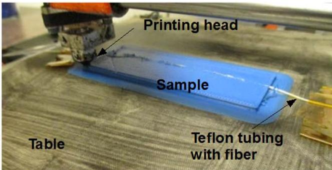
**FIGURE 3: SAMPLE BEING PRINTED FROM ABS TO TEST FIBER EMBEDDING METHODS.**
