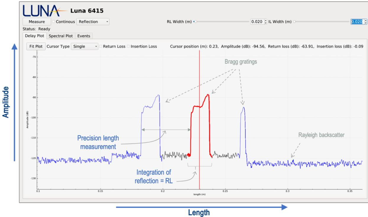
Figure 7. A scan of a Bragg gating string with a Luna 6415, connected in reflection, illustrates the high-resolution map of reflectance versus length, allowing high-precision measurement of RL, IL and path lengths
