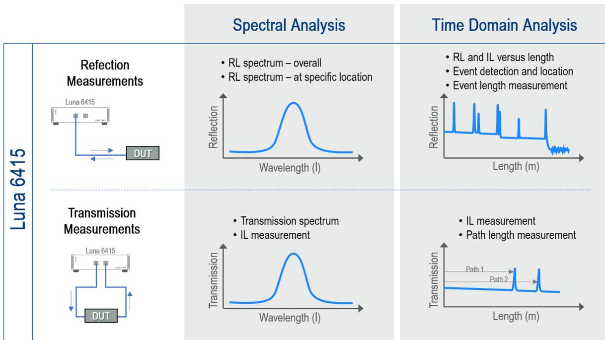
Figure 6. The Luna 6415 provides both traditional spectral analysis and time/length domain analysis of passive optical components; and is able to measure the loss of a DUT connected in reflection or in transmission
