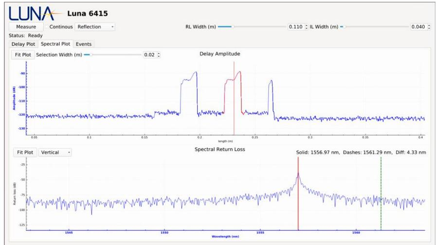
Figure 8. In the lower plot, the reflection spectrum of the second Bragg grating (selected and highlighted in red in the upper plot) is displayed
