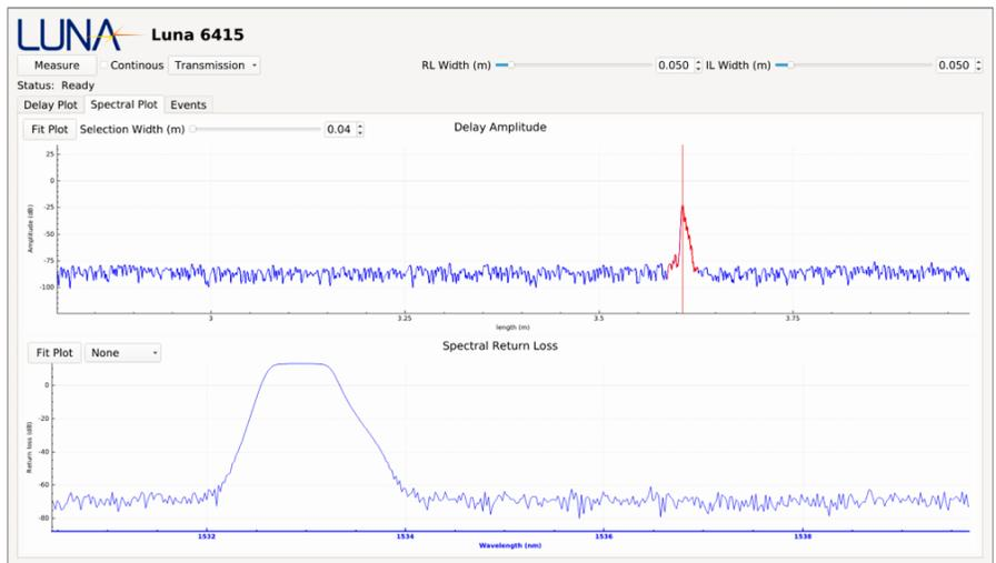
Figure 9. The transmission spectrum of an add-drop filter scanned by a Luna 6415 Lightwave Component Analyzer
