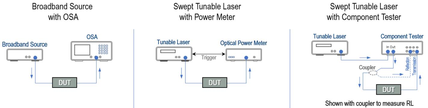
Figure 3. Traditional approaches to measuring component IL and RL with respect to wavelength
