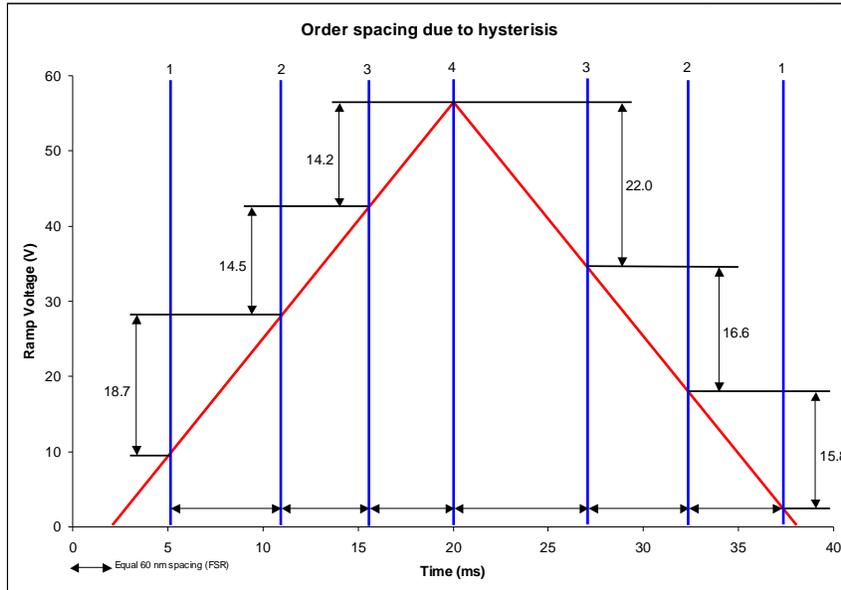
The filter resonance matches the input wavelength at each blue vertical line.
