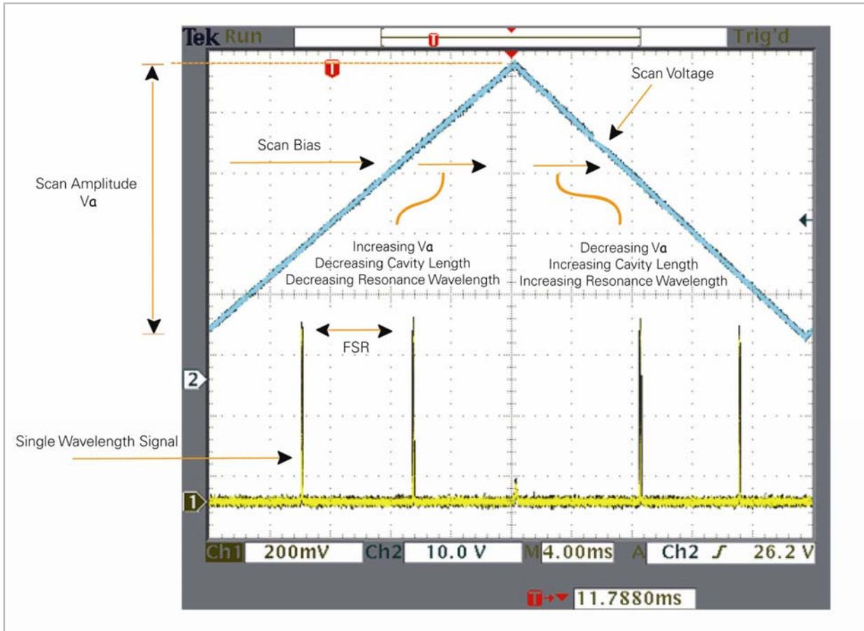
Note: This is a representative oscilloscope display of the scan voltage and the corresponding filter response.
