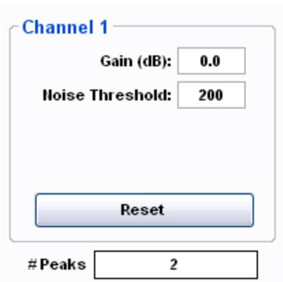
This group of controls is used to define the peak detection parameters for an x30 interrogator core, where peak detection is performed in the analog electronic circuitry of the interrogator. The resulting number of detected peaks for the channel is reported in the # Peaks indicator below the cluster.
