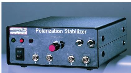
Fig. 5 The polarization stabilizer has an input port, an output port, and two device ports for accepting the two ends of a polarization sensitive device, such as a LiNbO<sub>3</sub> modulator. The stabilizer automatically adjusts the SOP to the modulator and ensures a maximum light transmission. The heart of the stabilizer is a fiber squeezer polarization controller.
