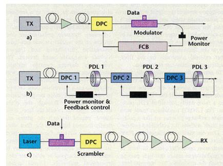
Fig. 3 Dynamic Polarization Controllers (DPC) for a) Polarization stabilization; b) PDL compensation; c) PDG mitigation.
