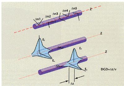
Fig. 1 A real fiber is like many retardation plates with different orientations and birefringences placed in serial. It is equivalent to a single retardation plate having a slow and fast axis and an equivalent birefringence. An optical pulse broadens because the two polarization components travel at different speeds.
