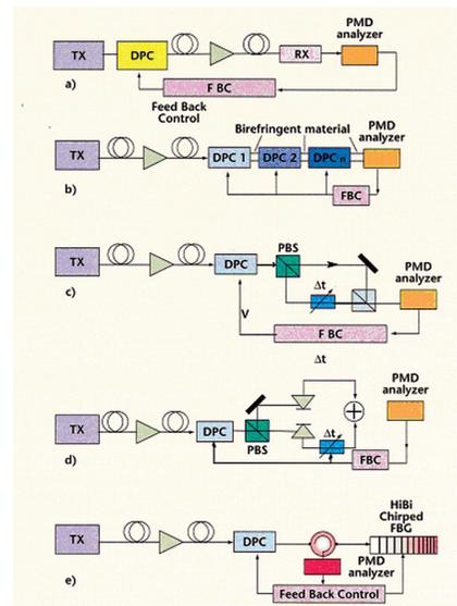
Fig. 2 Various PMD mitigation schemes: a) Principal state transmission method; b) Multiple retardation plates method; c) Optical delay line method; d) Electrical delay line method; e) Chirped HiBi fiber grating method. In all schemes, dynamic polarization controllers (DPC) having fast speed, low PDL, and low activation loss are required.
