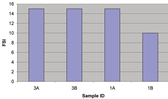
**Figure 3: ASTM E 162-02a Results for 0.3175 cm and 0.625 cm Pultruded Panels from Second Trial**
