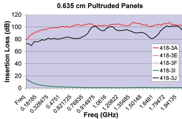
**Figure 5: ASTM D 4935-99 Results for 0.635 cm Pultruded Panels from First and Second Trials**
