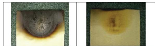
**Figure 2: Left—Front face of panel after 1 minute exposure to inner cone of propane torch. Right—Back face of panel after 1 minute exposure to inner cone of propane torch.**
