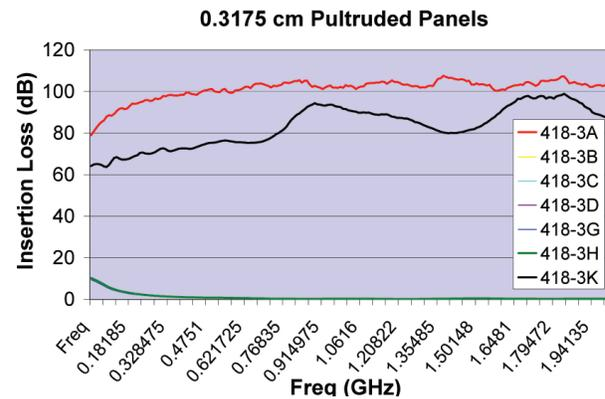
**Figure 4: ASTM D 4935-99 Results for 0.3175 cm Pultruded Panels from First and Second Trials**
