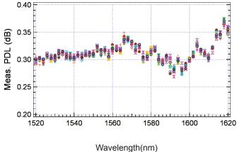
Figure 3. Wavelength scan and multiple (12) scan repeatability
