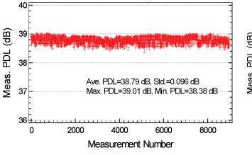
Figure 2. Measurement of high PDL sample: Polarizer
