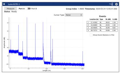
The OBR 6235 maps reflection versus length with high resolution, automatically detecting RL reflection events and IL locations that exceed user defined thresholds.
