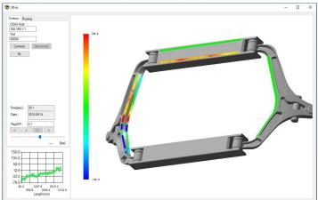
The ODISI 2D and 3D Visualization Software displays real-time data, as well as previously recorded data on 2D images or 3D models, which can be manipulated and moved to visualize different perspectives.
