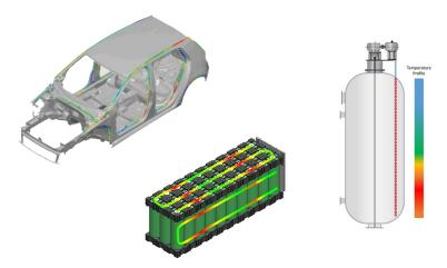
Instrumenting an automotive frame, battery pack or distillation column with highdefinition strain or temperature sensors yields comprehensive data and increased insight for model verification, testing and monitoring.
