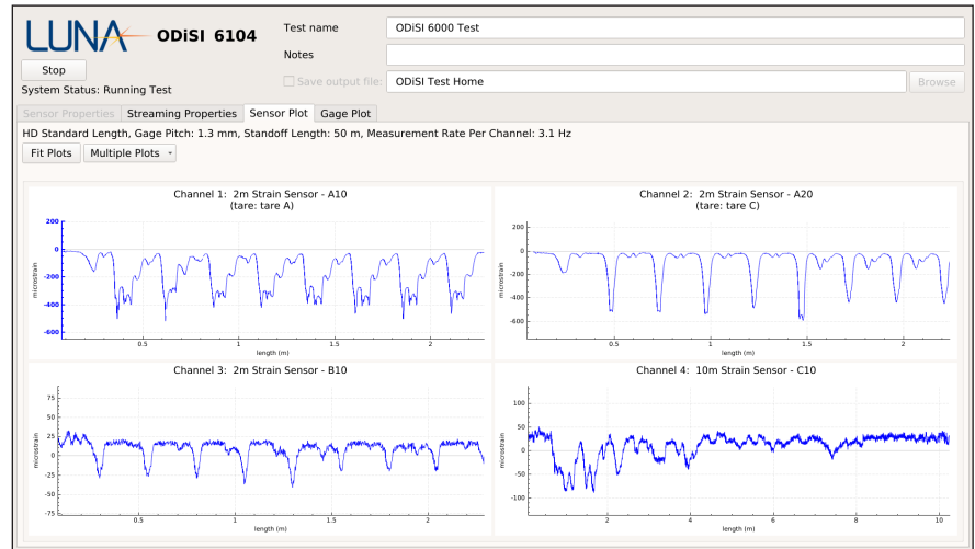
Multichannel sensor plot (strain/temperature versus length) in the ODiSI software.
