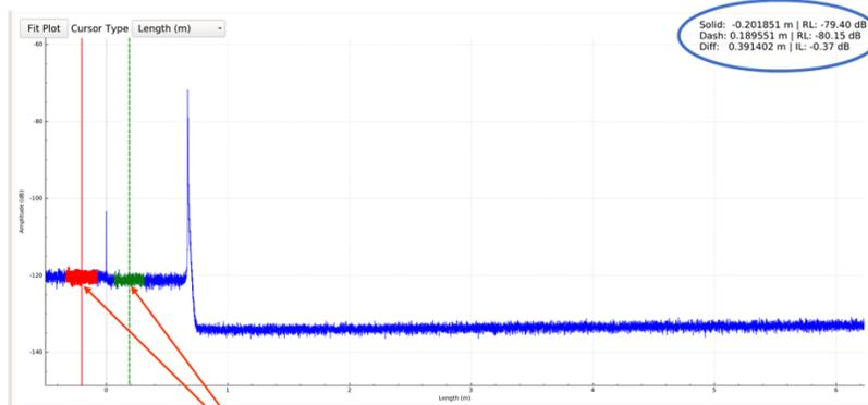
Compare the Rayleigh scatter on either side of the loss event by integrating under the colored sections of data. From this calculate one-way Insertion Loss (Differential Loss).
