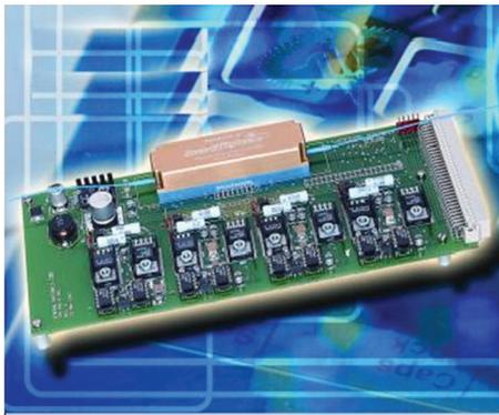
Fig. 2 A polarization scrambler board made with fiber squeezers
